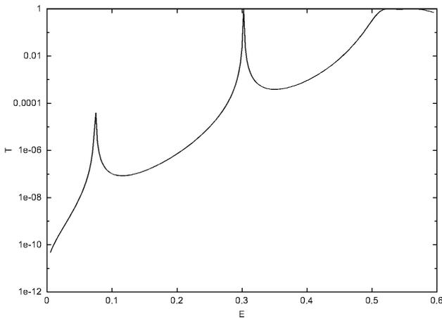
FIGURE 2. Plot of the transmission coefficient for a  $\text{Al}_{0.45}\text{Ga}_{0.55}\text{As}/\text{GaAs}$  DBRT structure with 5 nm barriers and a 5.5 nm GaAs well. The energy is given in eV.
