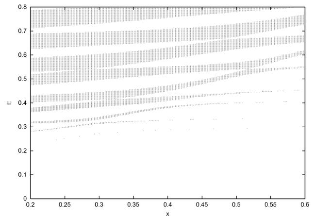
FIGURE 4. Electronic band structure as function of the Al concentration  $x$ , of the first barrier in Fig. 1. The energy is in eV.
