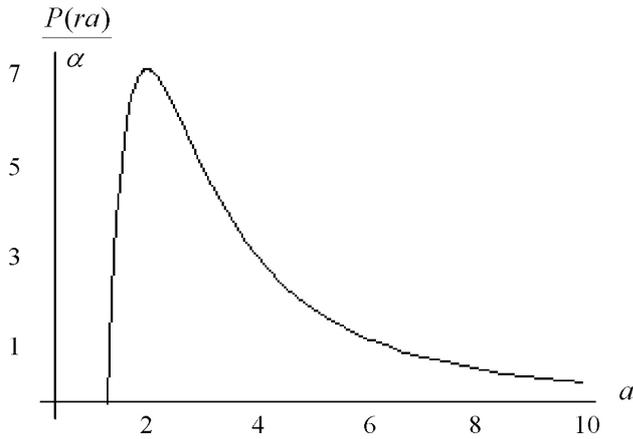
FIGURE 3. Performance of cooling power  $P(ra)/\alpha$  when  $a \rightarrow \infty$  and  $r = 0.9$ .
