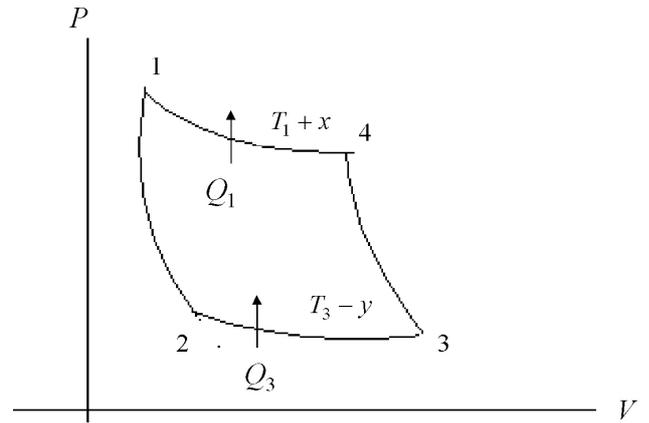
FIGURE 1. Inverse Carnot cycle like a refrigerator engine working at cool temperature  $T_3 - y$  and hot temperature  $T_1 + x$ .
