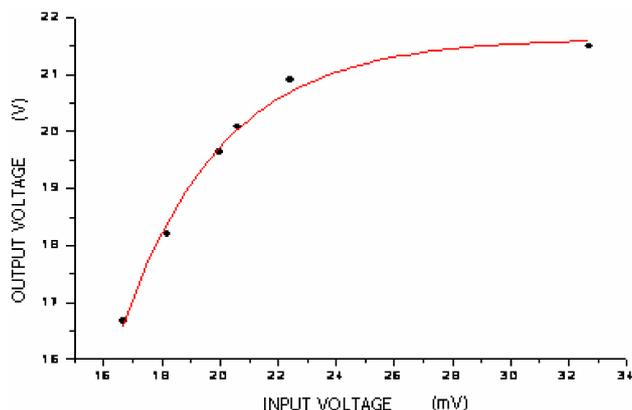
FIGURE 7. Input-Output plot obtained with the electronic system. This is qualitatively similar in gain to that obtained experimentally using the laser system. The continuous line shows the best fitting to the solution of a logistic equation.
