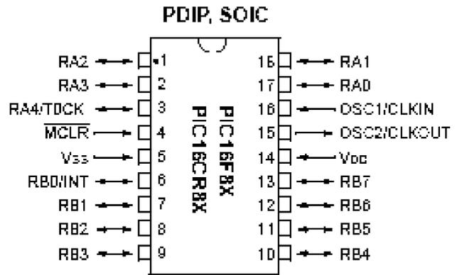
FIGURE 3. Schematic diagram of the microcontroller PIC16F84.
