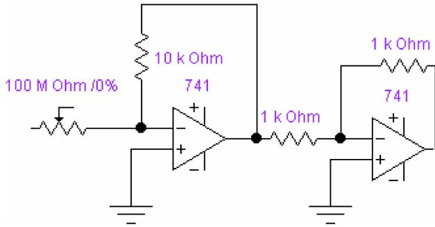
FIGURE 4. Inverting operational amplifiers used after the D-A converter in order to produce the electronic signal which represents the optical pulse produced by the laser oscillator.
