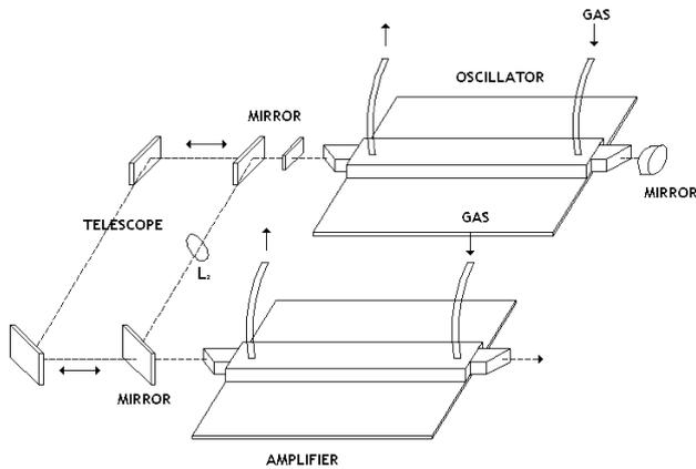
FIGURE 1. Schematic diagram of the oscillator-amplifier laser system built showing the optical delay line required to optimize the output power.
