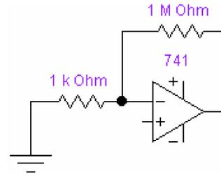
FIGURE 5. Electronic representation of the laser amplifier.
