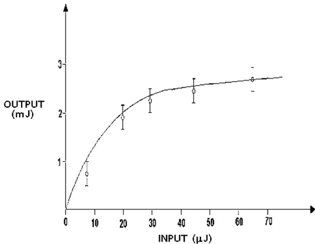
FIGURE 2. Input-output energy behavior of the laser amplifier. Points show the experimental data of the energy pulses produced by the oscillator (input) which are introduced into the amplifier, as well as the energy of the same pulses at the end of the amplifier (output). The continuous line shows the best fitting to the solution of a logistic equation.
