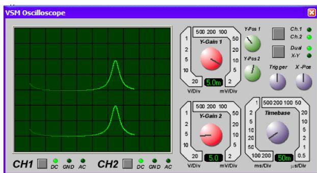
FIGURE 8. Oscilloscope results showing, in the upper part, the electronic signal which represents the optical signal produced by the laser oscillator and, in the lower part, the electronic signal which represents the amplified optical signal. Vertical voltage scales show a gain of 1000.
