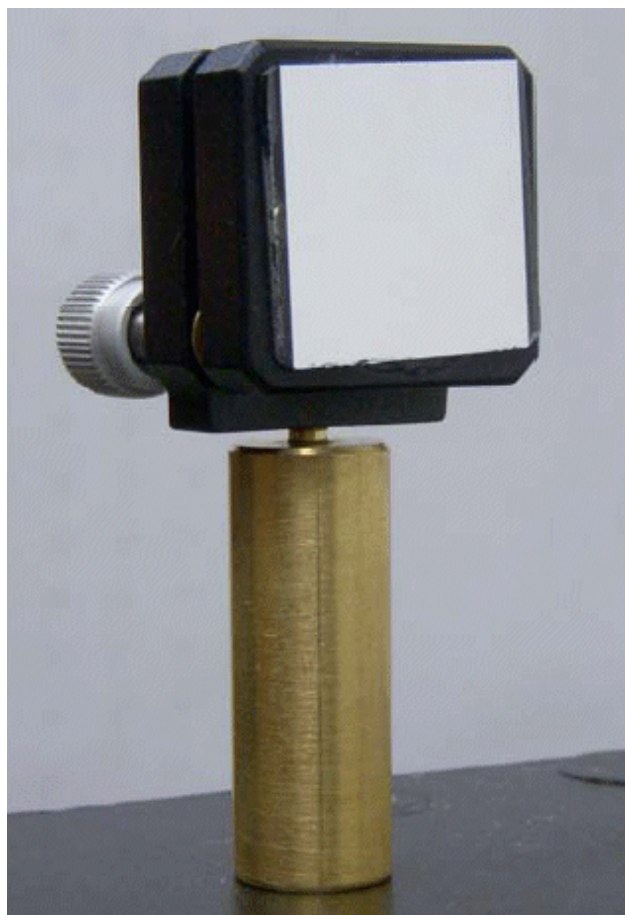
FIGURE 2. Mirror on a movable mount with two adjusting knobs and support post (LABEL B).
