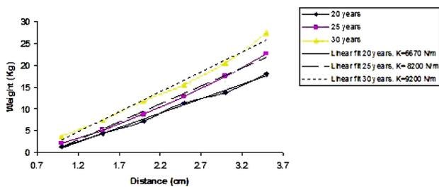
FIGURE 3. Applied force on human thorax vs. compression distance for 20, 25, and 30 years old men. Values of the elastic constants of the law of Hooke's law are also shown.
