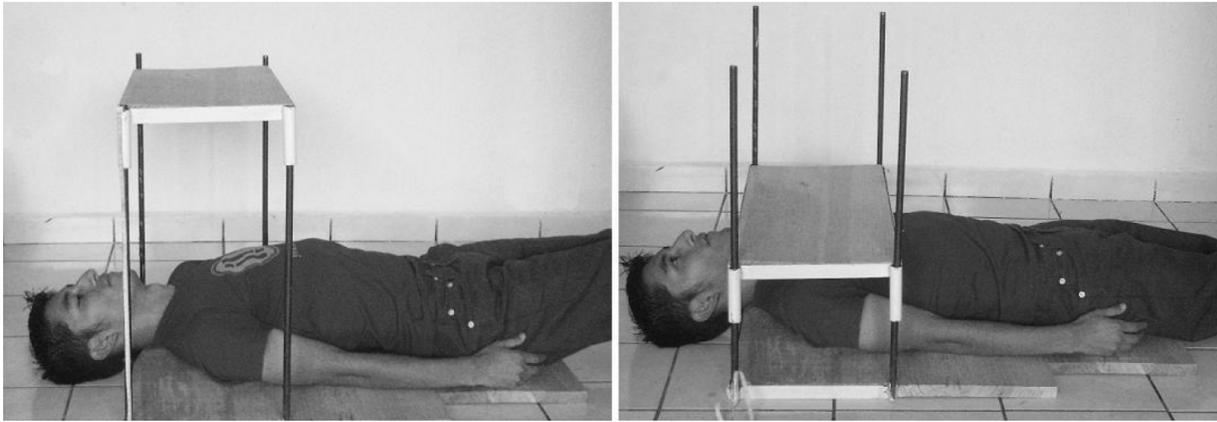
FIGURE 2. Device used to measure the compression of the thorax under vertical stress. Different weights were positioned on the horizontal platform.
