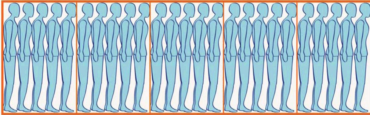
FIGURE 6. Schematic diagram of a crowded divided container. The three divisions separating sets of five people are built in order to decrease cumulative inertial forces.
