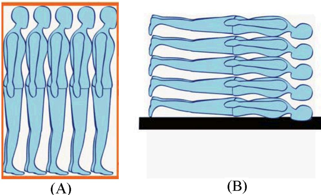
FIGURE 1. Panel (A): Schematic diagram of a crowded container with five people standing-up. Panel (B): Same people but stacked horizontally in a gravitational field. If the container in (A) experiences braking or decelerations in the right direction, then forces on people inside in the container are analogous to vertical gravitational forces suffered by stacked people.
