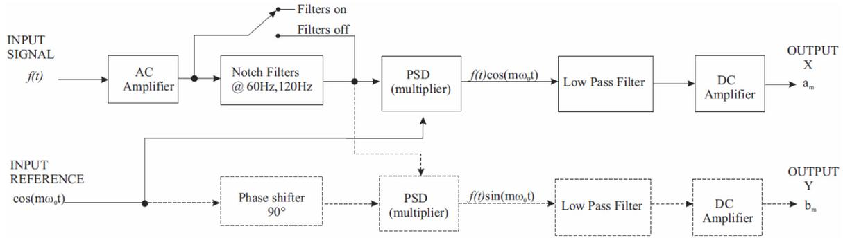
FIGURE 1. General block diagram of a lock-in (dual lock-in includes dashed blocks).
