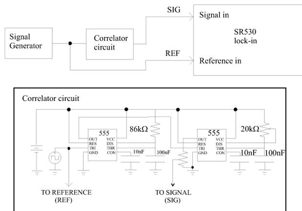
FIGURE 4. Experimental set up for measuring the Fourier coefficients of SIG.
