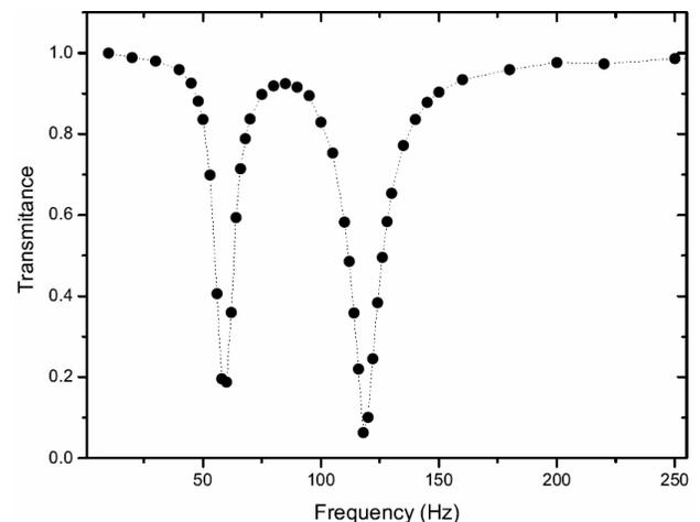
FIGURE 6. Transmittance of the Notch filters of the lock-in SR530.
