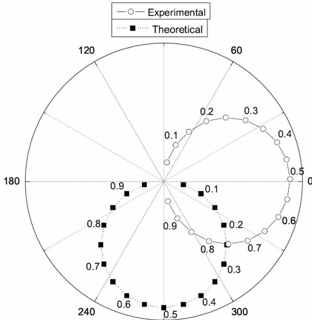
FIGURE 7. Experimental and theoretical polar plot of  $(a_1, \phi_1)$  as function of duty cycle  $\delta_s$ .
