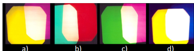
FIGURE 3. a) Yellow and Magenta; b) to d) Experimental results of mixing complementary colors to obtain white light.
