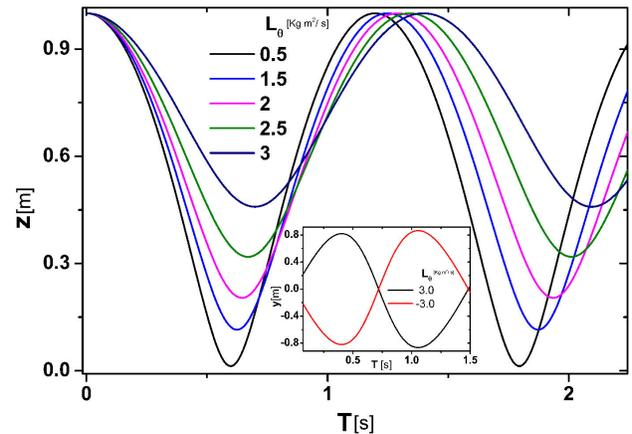
FIGURE 1. The system **A**, the free fall height  $z$  as a function of time for different values of angular momentum  $L_\theta$  and with parameters  $n = 2$ ,  $r(0) = 1.0 \text{ m}$ ,  $\dot{r}(0) = 0 \text{ m/s}$ ,  $\theta(0) = 0.0 \text{ rad}$ . The inset shows the case of a negative value of angular momentum on the  $y$ -axis.
