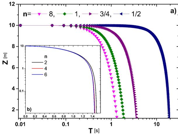
FIGURE 5. The system **B**, a) Shows the the fall height  $z$  as a function of time for different values of the exponent  $n$  in the Eq. 1) and the parameters  $r(0) = 10.0 \text{ m}$ ,  $\dot{r}(0) = 0 \text{ m/s}$ . b) Is the same but for other values of  $n$ .
