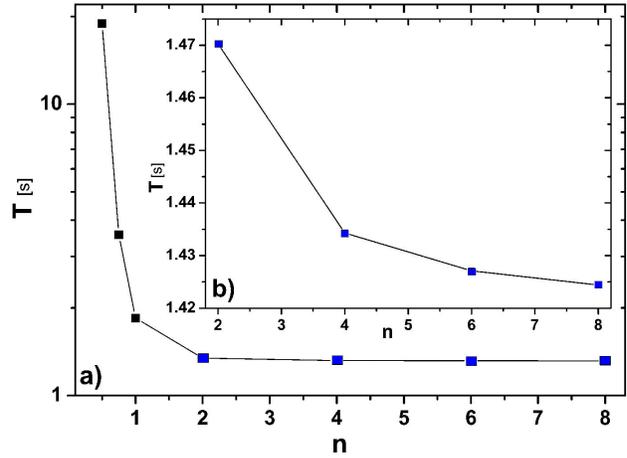
FIGURE 6. The system **B**, a) Shows the free fall time as a function of the value of  $n$  in the equation of the cone (1), with parameters  $r(0) = 10.0 \text{ m}$ ,  $\dot{r}(0) = 0 \text{ m/s}$ . b) Shows a zoom for the last four points.
