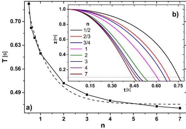
FIGURE 4. The system **A**, a) shows the free fall time as a function of the value of  $n$  in the equation of the cone, with parameters  $L_\theta = 0.01 \text{ kg m}^2/\text{s}$ ,  $r(0) = 1.0 \text{ m}$ ,  $\dot{r}(0) = 0 \text{ m/s}$ ,  $\theta(0) = 0.0 \text{ rad}$ . b) Shows the fall height  $z$  as a function of time for different values of the exponent  $n$  and the same parameters. The dotted line sets the cut-off distance  $z = 0.1 \text{ m}$ .
