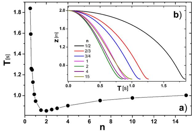
FIGURE 7. The system **A**, a) Shows the free fall time as a function of the value of  $n$  in the equation of the cone (1), with parameters  $r(0) = 2^{1/n} \text{ m}$ ,  $\dot{r}(0) = 0 \text{ m/s}$ , and for  $L_\theta$  use Eq. (15). b) Shows the fall height  $z$  as a function of time for different values of the exponent  $n$  in the equation of the cone.
