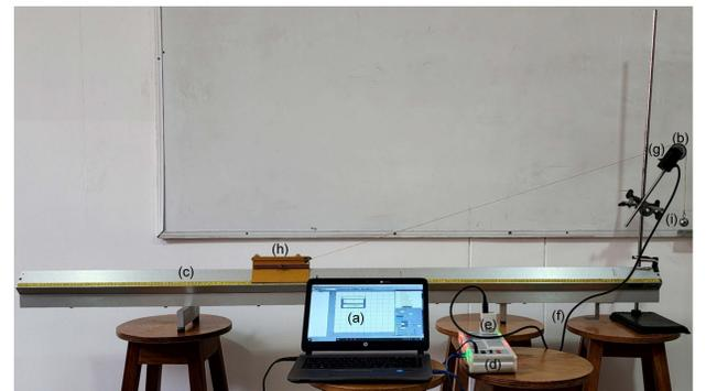
FIGURE 3. Experimental configuration: (a) computer; (b) combination spoked wheel [19]; (c) air track [20]; (d) sensor CASSY 2 [21]; (e) timer S [22]; (f) multi-core cable, 6 poles, 1.5 m [23]; (g) combination light barrier [24]; (h) mass  $m_1$ , and (i) mass  $m_2$ .
