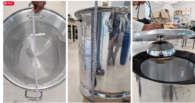
FIGURE 1. Photo of the detector at the moment of assembly. The liquid scintillator and the PMT are clearly visible. The PMT is the model Electron Tubes 9354KB with a diameter of 200 mm. The cylindrical steel container has a diameter of 52 cm and it is filled with liquid scintillator up to a height of 45 cm.
