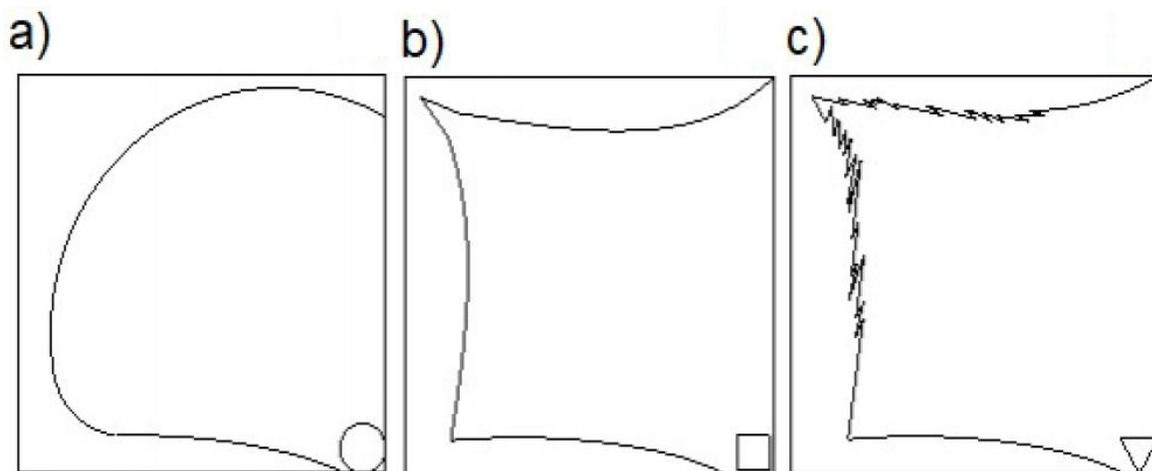
FIGURE 3. Profiles generated with different kind of spacers. a) Profile with circular spacer. b) Profile with square spacer. c) Profile with triangular spacer.
