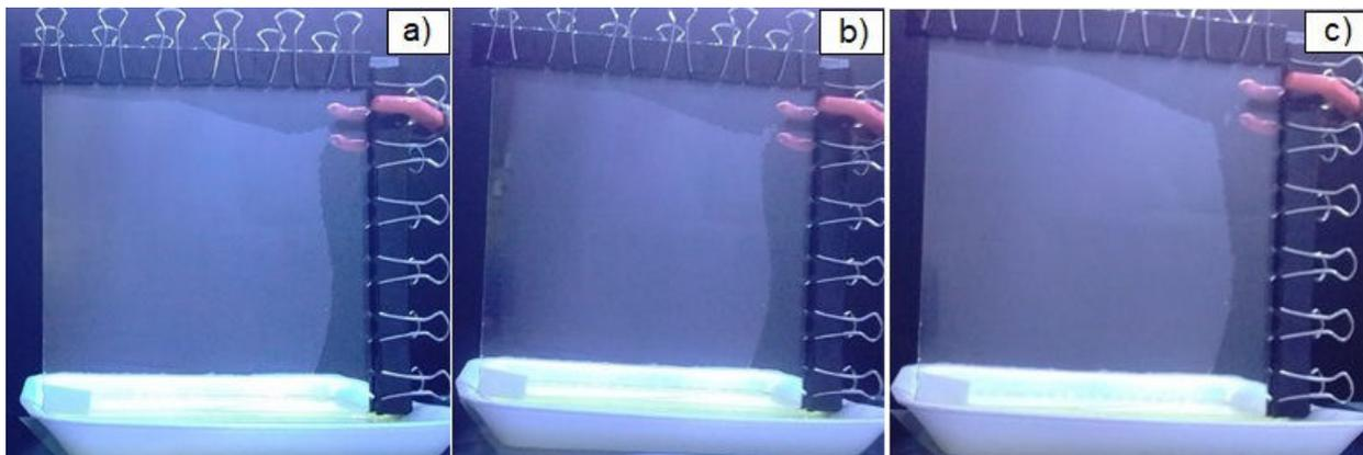
FIGURE 9. Change in the spacer. Opening angle:  $3.08^\circ$ . Opening geometry: square. a) Profile generated in 24 hours. b) Profile generated in 48 hours. c) Profile generated in 72 hours.
