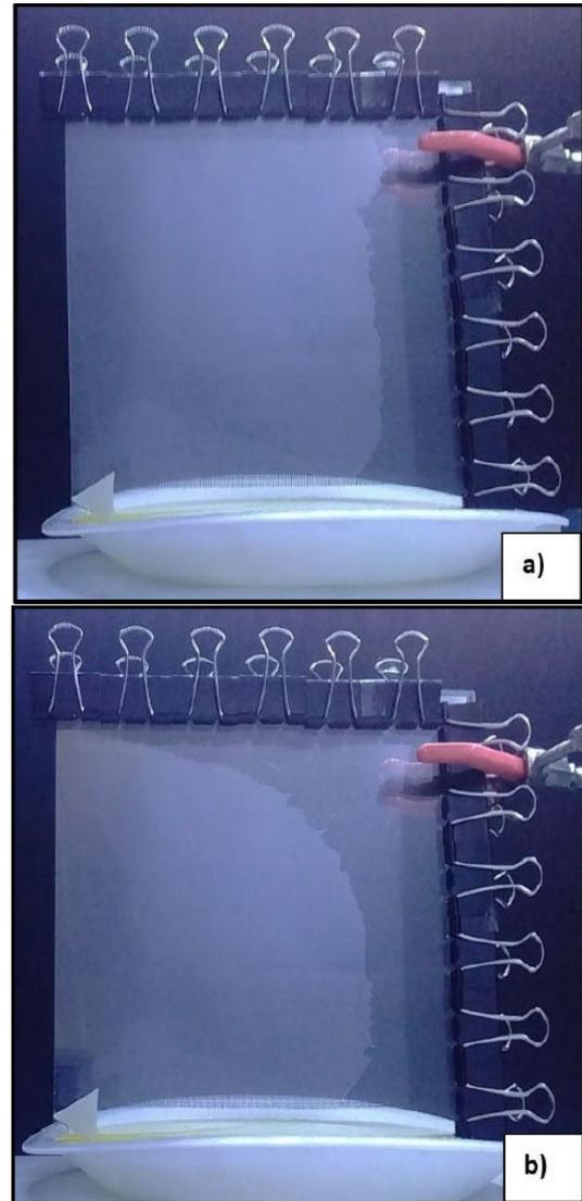
FIGURE 12. Profile generated with triangular spacer. a) Generated profile after 96 hours. b) Generated profile when the fluid is in an equilibrium position.
