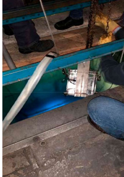
FIGURE 9. Introducing the detector system inside the gamma irradiator pool, by means of a system of cables and pulleys.
