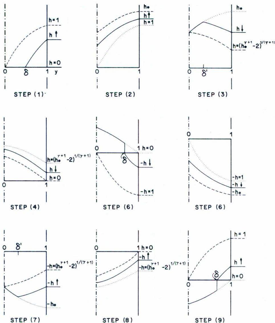
Fig. 6 Schematic representation of the normalized internal field distribution for the different stages of the magnetization cycle for the case when  $2^{1/(\gamma+1)} \leq h_0 < h_{c2}$ . (Because of the symmetry only one half of the cylinder is shown). In each one of the step figures the dotted line represents the initial state, the dashed line the final state and the full line an intermediate state.
