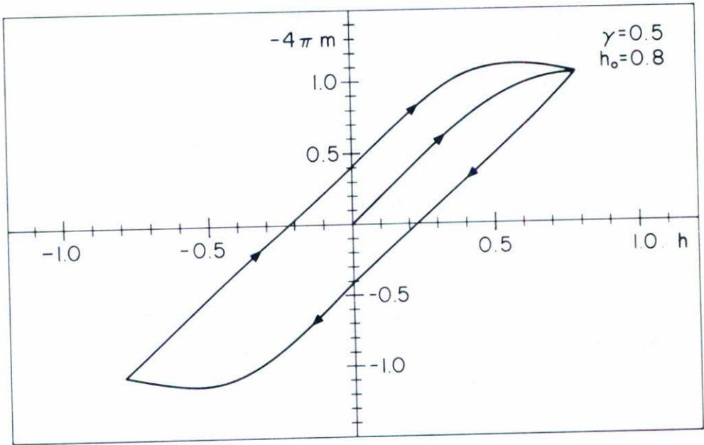
Fig. 3 Normalized magnetization cycle curve for  $\gamma = 0.5$  and  $h_0 = 0.8$ .
