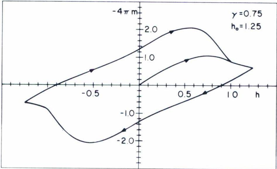
Fig. 5 Normalized magnetization cycle curve for  $\gamma = 0.75$  and  $h_0 = 1.25$ .
