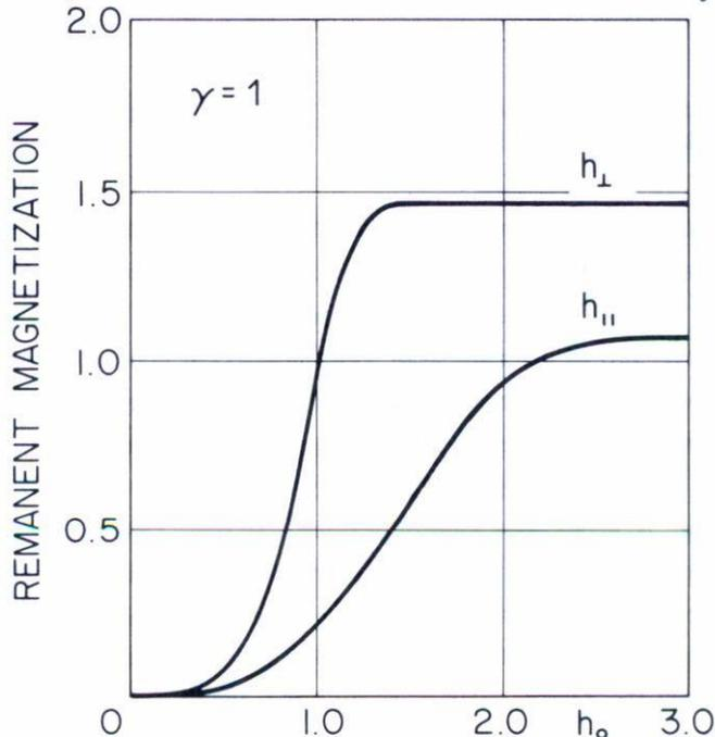
Fig. 9 The normalized remanent magnetization as a function of  $h_0$  for the perpendicular and parallel cases when  $\gamma=1.0$ .
