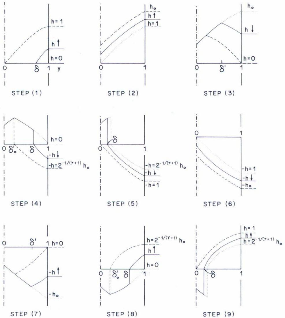
Fig. 4 Schematic representation of the normalized internal field distribution for the different stages of the magnetization cycle for the case when  $1 \leq h_0 \leq 2^{1/(\gamma+1)}$ . (Because of the symmetry only one half of the cylinder is shown). In each one of the step figures the dotted line represents the initial state, the dashed line the final state and the full line an intermediate state.
