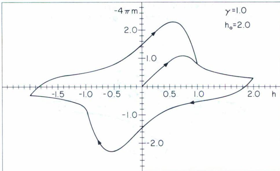
Fig. 7 Normalized magnetization cycle curve for  $\gamma = 1.0$  and  $h_0 = 2.0$ .
