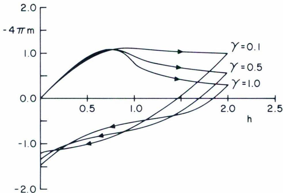
Fig. 10 Three normalized magnetization curves, corresponding to  $\gamma = 0.1$ ,  $\gamma = 0.5$  and  $\gamma = 1.0$ .
