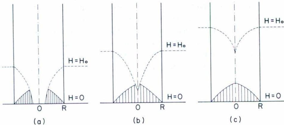
Fig. 1 Schematic representation of the three possible internal field distributions due to the remanent magnetic flux.
