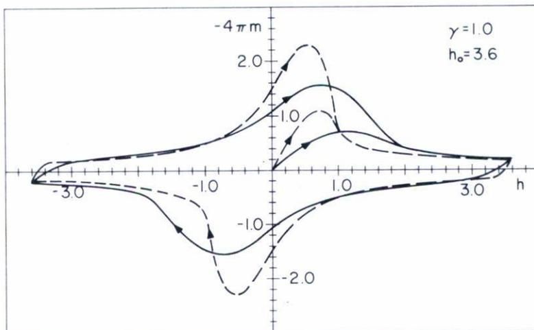
Fig. 8 Normalized magnetization cycle curve for the perpendicular (dashed line) and parallel (full line) cases when  $\gamma=1.0$  and  $h_0=3.6$ .
