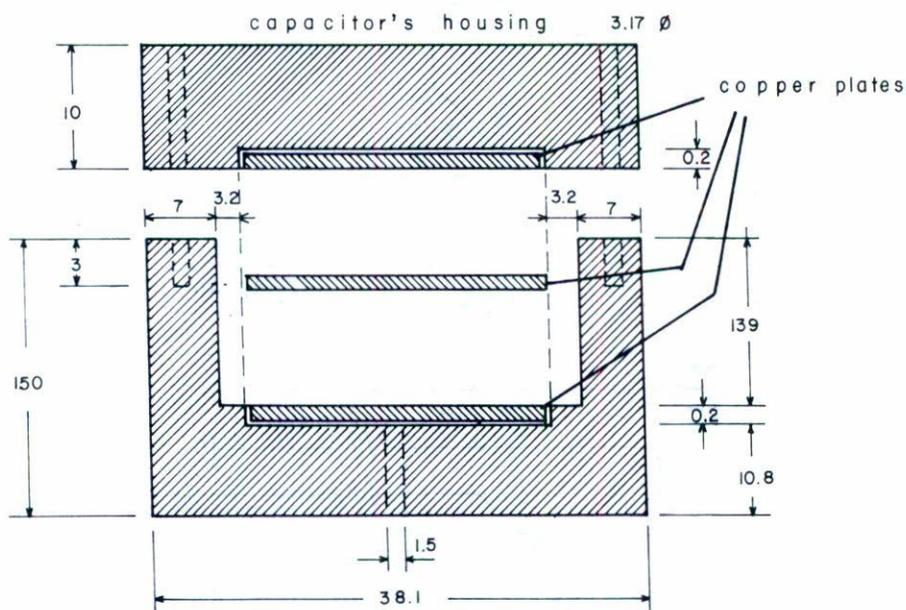
Fig. 4 Cross section of the transducer, all dimensions in mm. (Not to scale).
