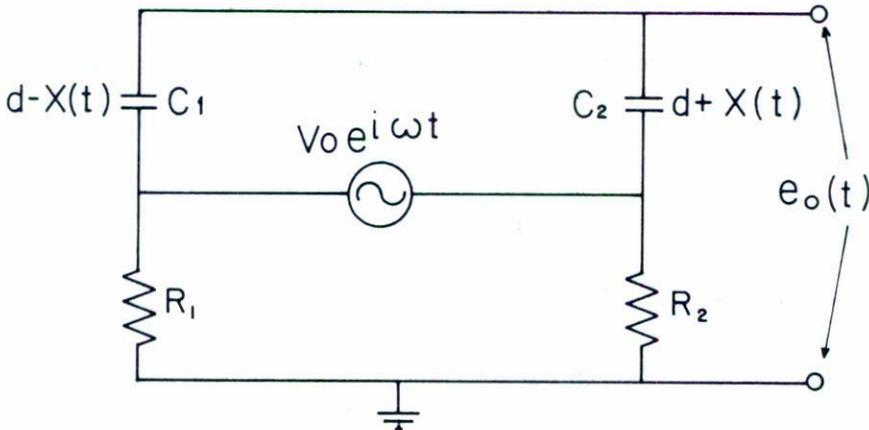
Fig. 2 Scheme adopted to obtain an output voltage  $e_o(t)$  from the capacitive transducer.
