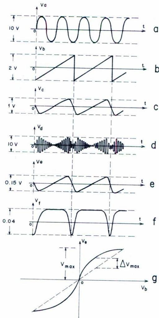
Fig. 6 Schematical representation of typical waveforms, responses and linearity in the experimental array. Representations not to scale.
