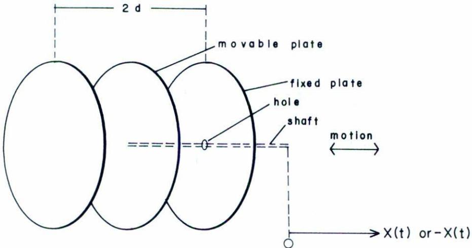
Fig. 1 Sketch of the capacitive transducer. Separation between fixed plates =  $2d$ . Displacement from midway position =  $-X(t)$  or  $+X(t)$ .
