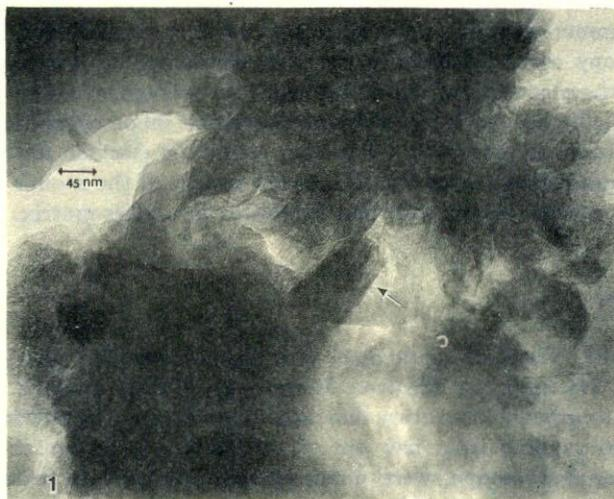
FIGURE 1. Low magnification TEM micrographs showing a rather large microcrystal in the amorphous structure of a silica glass sample. Notice the regular shape of the cristallites.
