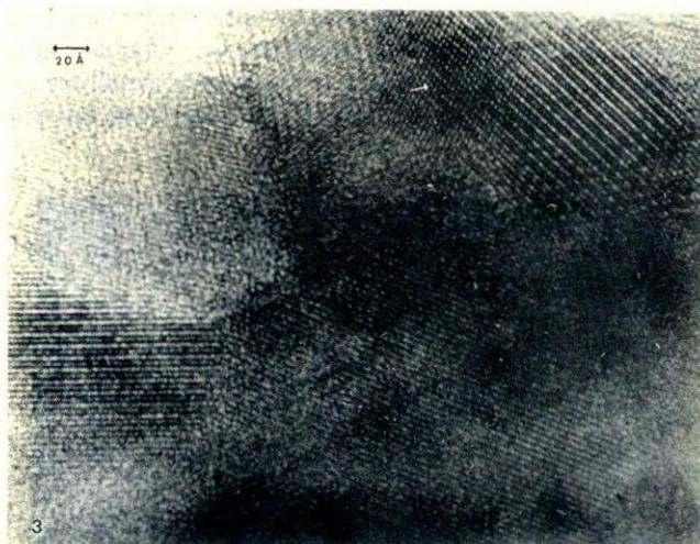
FIGURE 3. High Resolution micrographs showing the lattice structure of the tetragonal structure of a  $\alpha$ -cristobalite microcrystal embedded in the glass structure. The arrows point to some dots which correspond to the atomic arrangement of the  $\alpha$ -cristobalite.
