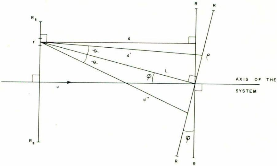
FIGURE 2. Element of source area located at distance  $r$  from the axis of the system. This same element can be assumed, however, to be located on the perpendicular axis of the detector window which (as seen from the location of the element of source area) appears to be rotated by an angle  $\phi$ .
