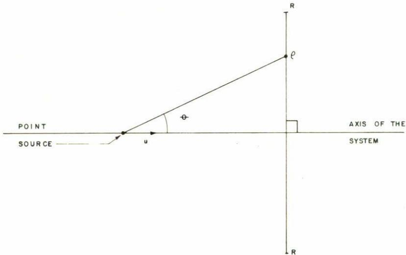
FIGURE 1. Point source located on the perpendicular axis of the detector window of radius  $R$ .
