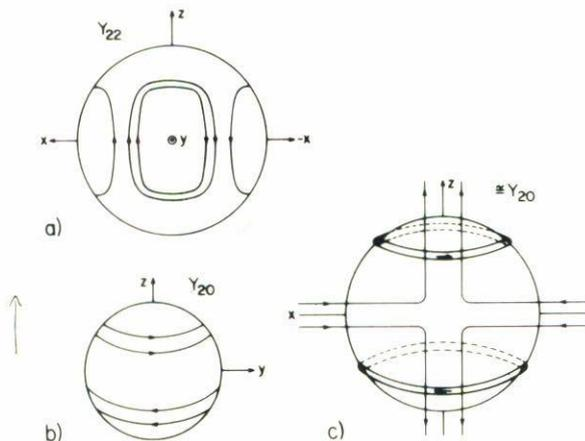
FIGURE 3. Typical streamlines on the surface of a sphere: a) generated by  $Y_{22}(\theta, \phi) = c$ . b) By  $Y_{20}(\theta, \phi) = c$ . c) Shows the experimental set up for a quadrupole trap with 2 coils at  $\pm 45^\circ$  and currents flowing in opposite directions. The dominant component for this trap is  $Y_{20}$ .
