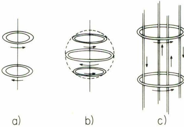
FIGURE 1. Various configurations of magnetic traps for neutral atoms; a) quadrupole, b) octupole and c) hybrid, which is a mixture of a uniform axial field, and octupole and a transverse quadrupole.
