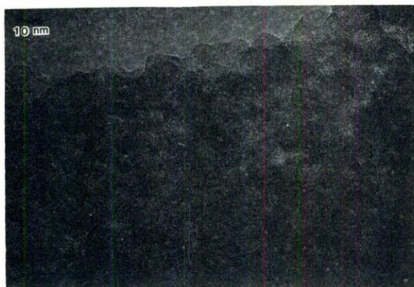
FIGURE 7. TEM image of a gel sample fired at 800°C. Notice that the necking is more visible as compared with the previous samples.
