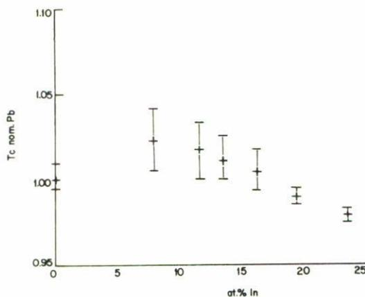
FIGURE 3. Normalized superconducting transition temperature as a function of the atomic percent of In in Pb. The spreads shown are transition widths, not experimental errors.
