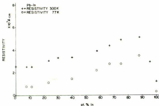
FIGURE 2. Electrical resistivity as a function of In concentration for Pb-In alloys, both at room temperature and at 77 K.
