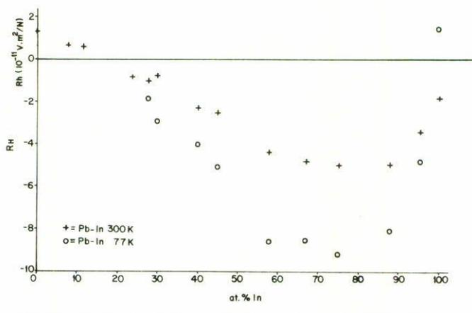
FIGURE 1.  $R_H$  as a function of In concentration for Pb-In alloys, both at room temperature and at 77 K.
