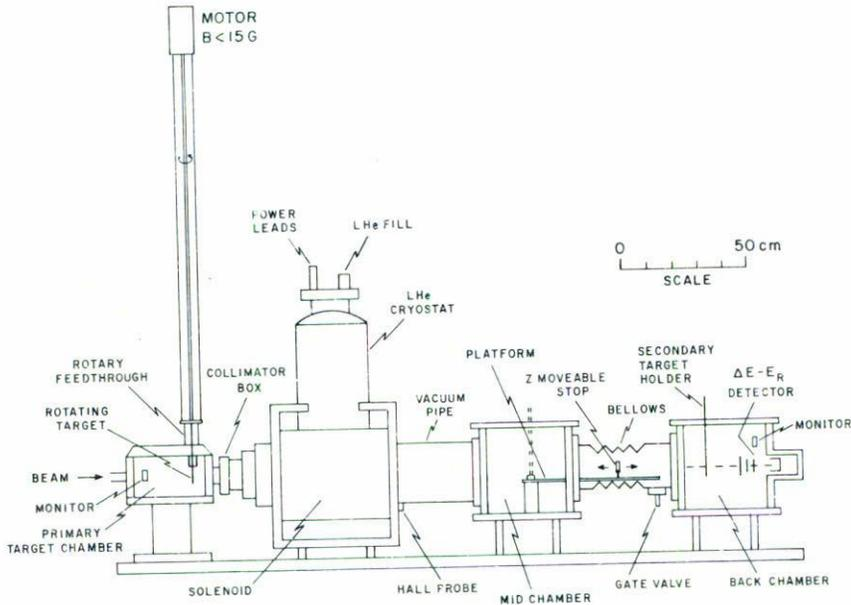
FIGURE 1. Schematic diagram of the RNB beamline. Note in particular the rotating target mechanism, with its motor placed well outside the fringe field of the solenoid, and the  $z$ -moveable stop used to remove inelastically scattered primary beam particles from the secondary beam.
