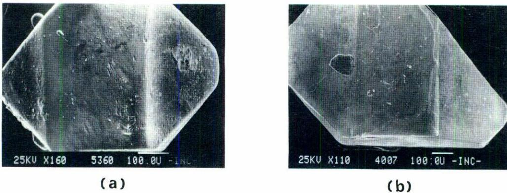
FIGURE 5. Photomicrographs of KDP single crystals showing (a) surface morphology and (b) typical habit with prismatic and pyramidal faces.
