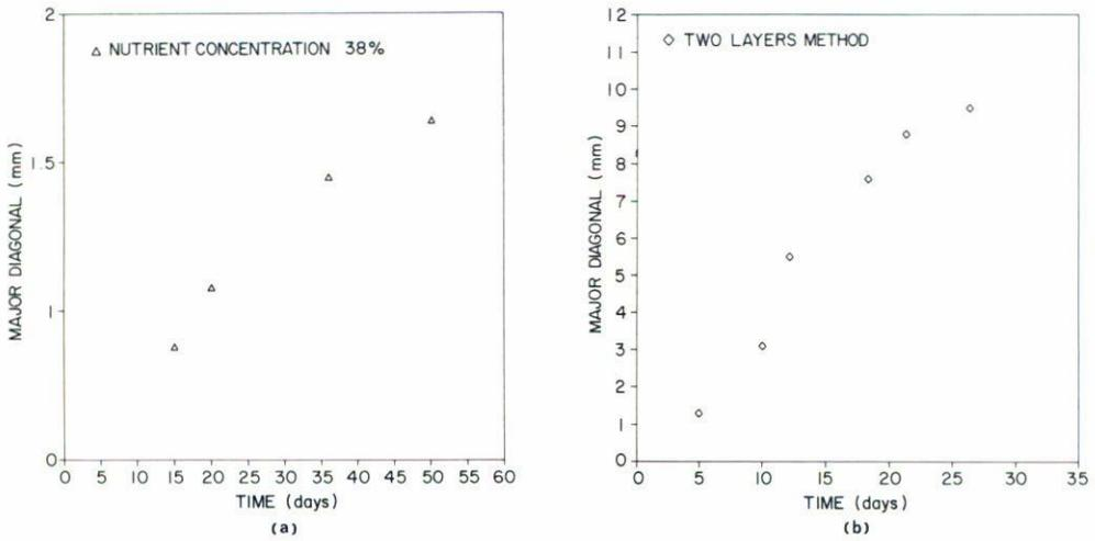
FIGURE 2. Growth rate measurements for (a) calcite and (b) KDP crystals.
