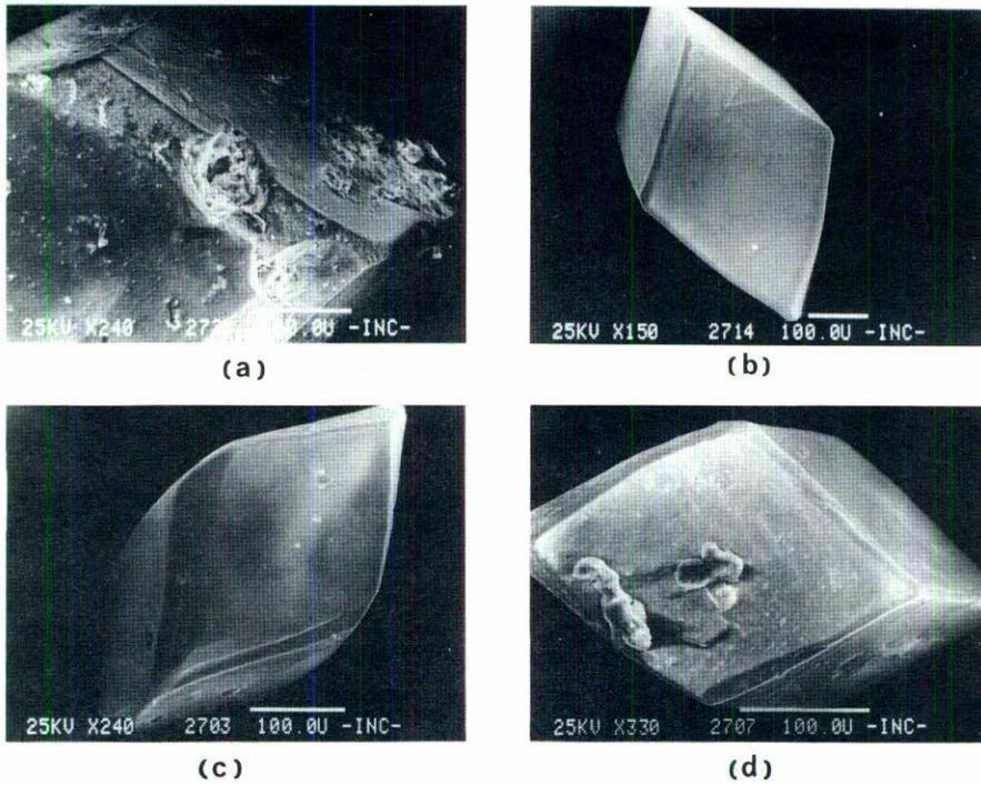
FIGURE 4. SEM micrographs of calcite crystals. (a) and (b) surface morphology for crystals grown with 30% and 38% of nutrients, respectively. (c) and (d) show crystals grown adding small quantities of NaOH to the nutrients 38% concentrated.
