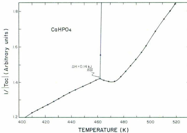
FIGURE 2. Ac-calorimetric heating curve,  $1/|T_{ac}|$ , which is proportional to the heat capacity,  $C_P(T)$ , in the 400–530 K temperature range, for a  $\text{CaHPO}_4$  sample. The solid line is drawn as a guide to the eye.
