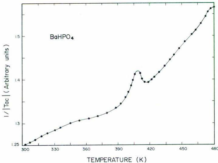
FIGURE 3. Ac-calorimetric heating curve,  $1/|T_{ac}|$ , in the 300–500 K temperature range, for a  $\text{BaHPO}_4$  sample. Full curve is guide to the eye.
