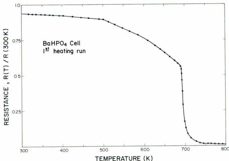
FIGURE 4. Relative resistance,  $R(T)/R(300\text{ K})$ , of a  $\text{BaHPO}_4$  cell on a first heating run in the 300–800 K temperature range. Full curve is guide to the eye.
