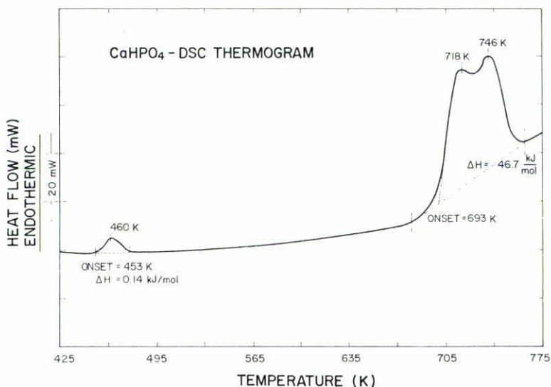
FIGURE 1. DSC heating curve for a freshly prepared CaHPO<sub>4</sub> sample. The transition points are 453 K and 693 K, respectively. The heating rate is 10 K/min.
