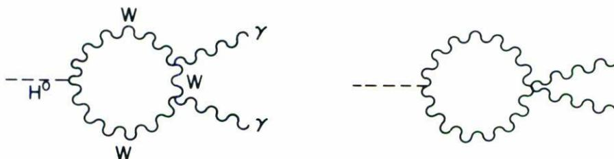
FIGURE 1. Dominant Feynman diagram contributing to  $\Gamma(H^0 \rightarrow \gamma\gamma, \gamma Z)$ .
