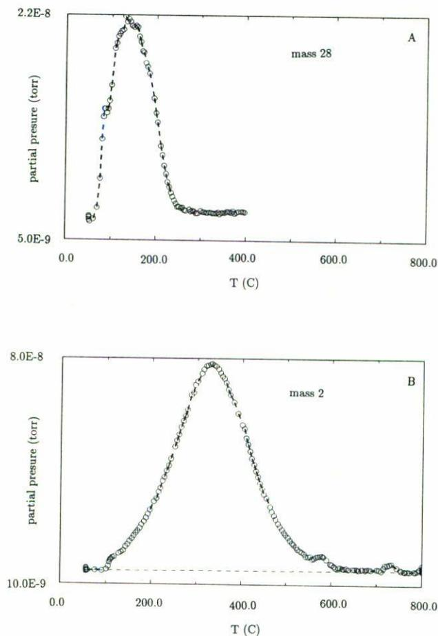
FIGURE 5. TDS spectra for: a) CO desorption from Pd foil after exposure to 500 L of CO and using a heating rate of 10 degree/s; and b) H<sub>2</sub> desorption after exposure to 500 L H<sub>2</sub> and using a heating rate of 5 degree/s.
