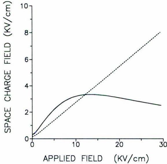
FIGURE 1. Dependence of the space charge field amplitude on the applied field with experimental parameters as given in Table I (with  $\Lambda = 2.4 \mu\text{m}$ ,  $N = 10^{17} \text{cm}^{-3}$ ). Present work and Ref. [13]: are coincident and given by —; Ref [7]: - -.
