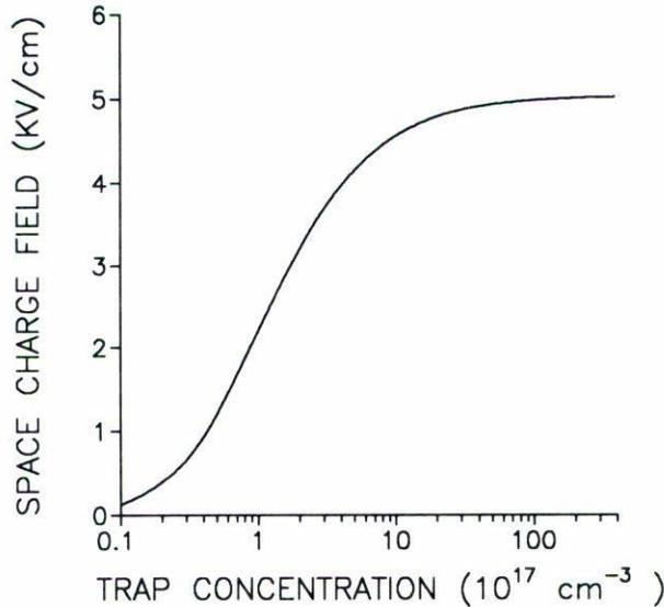
FIGURE 3. Dependence of the amplitude of the space charge field on trap concentration ( $E_a = 5.0$  KV/cm,  $\Lambda = 2.4$   $\mu$ m). Experimental parameters as in Table I.
