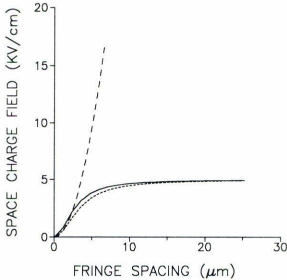
FIGURE 2. Dependence of the space charge field amplitude on the grating spacing (with  $E_a = 5.0$  KV/cm,  $N = 10^{17}$  cm $^{-3}$ ). Present work: —; Ref. [13]: - - - ; Ref. [7]: - · - ·. Experimental parameters are as given in Table I.
