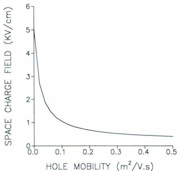
FIGURE 4. Influence of hole mobility on the amplitude of the space charge field ( $E_a = 5.0$  KV/cm,  $N = 10^{17}$  cm<sup>-3</sup>,  $\Lambda = 2.4$   $\mu$ m). Experimental parameters as in Table I.
