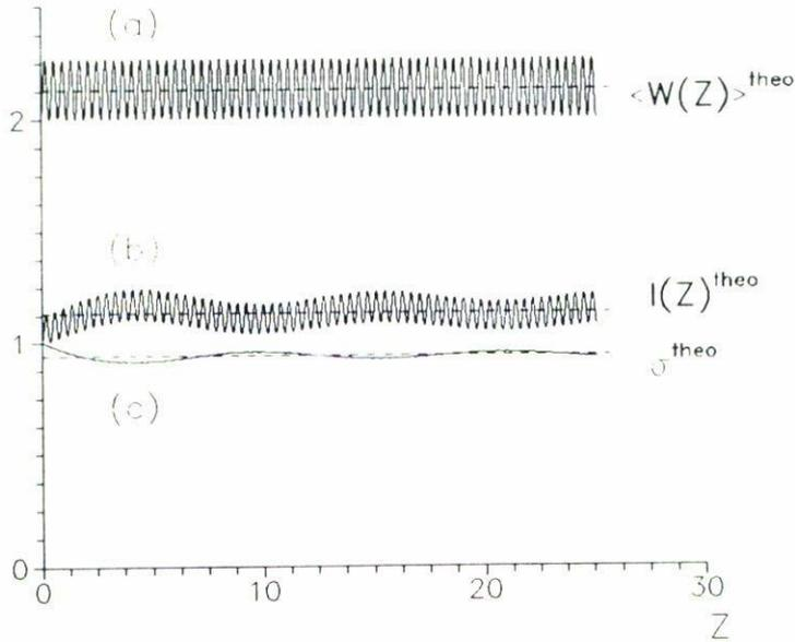
FIGURE 7. Spatial traces of (a) the energy, (b) the peak intensity, and (c) the width of a pulse propagating through a fiber possessing the periodical gain profile of Fig. 1b, with  $g_0 = 1$  and  $L = Z_0/4$ . The theoretically predicted parameters are indicated by the corresponding horizontal lines.
