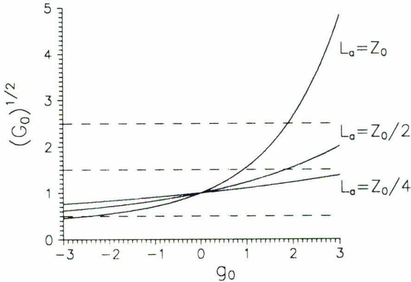
FIGURE 3. Behavior of  $\sqrt{G_0}$  for the gain profile of Fig. 1a. The three curves corresponds to the amplification lengths indicated in the figure in soliton units. According to Eq. (1), a soliton period  $Z_0$  corresponds to a distance  $Z = \pi/2$ .
