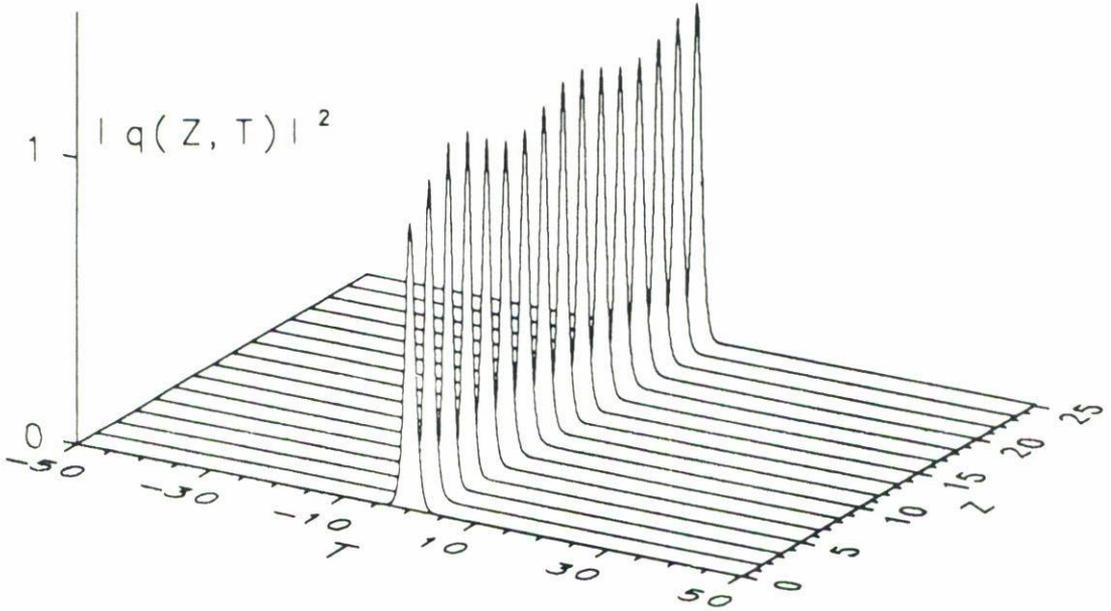
FIGURE 5. Temporal behavior of an initial first order soliton as it propagates through a fiber possessing the periodical gain profile of Fig. 1b with  $g_0 = 1$  and  $L = Z_0/2$ . The total propagation distance is  $32L$ , and each curve is taken at the distance interval of  $2L$ .
