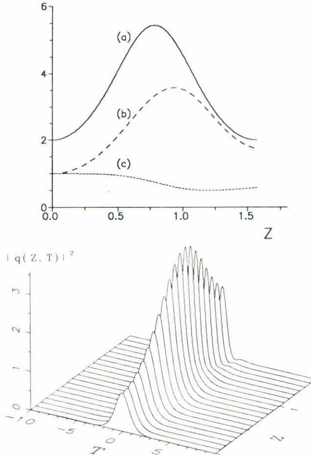
FIGURE 2. Propagation of an initial first order soliton through the first period of the gain profile of Fig. 1b, with  $g_0 = 2$  and  $L = \pi/2 = Z_0$ . In (a) we show the temporal pulse evolution and in (b) the spatial evolution of the pulse energy,  $W(Z)$ , the pulse peak intensity,  $I_p(Z)$  and the pulse width,  $\sigma(Z)$ .
