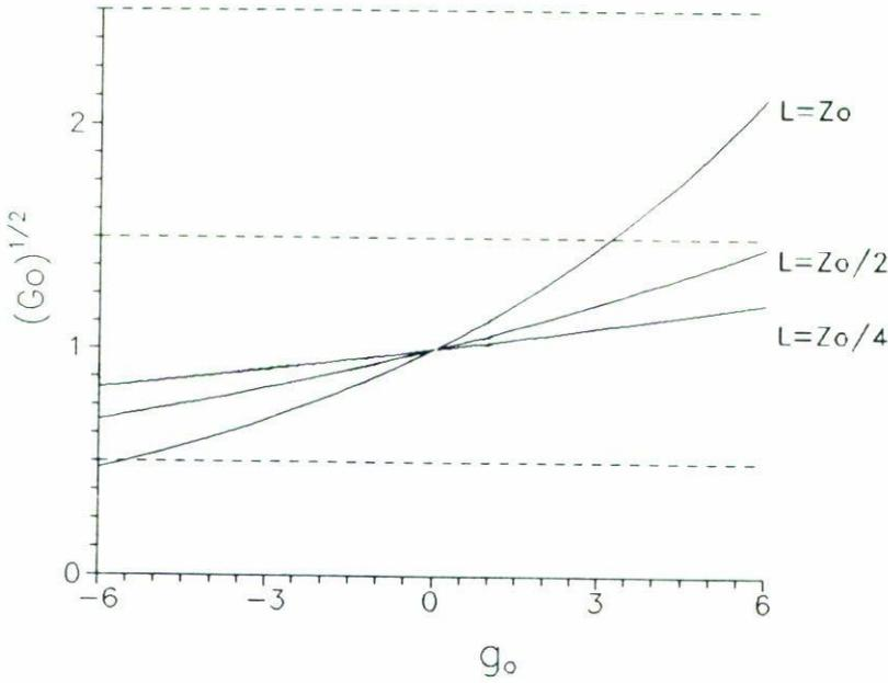
FIGURE 4. Behavior of  $\sqrt{G_0}$  for the sinusoidal gain profile of Fig. 1b. The three curves correspond to the period lengths indicated in the figure in soliton units.
