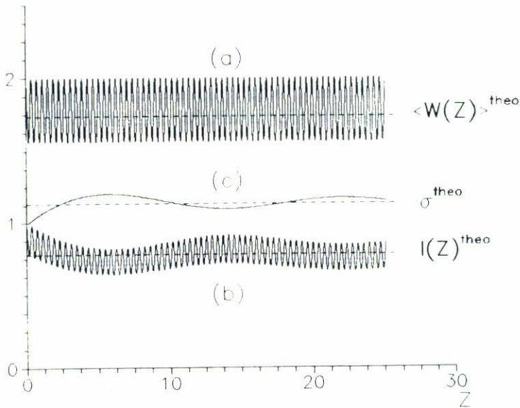
FIGURE 8. Spatial traces of (a) the energy, (b) the peak intensity, and (c) the width of a pulse propagating through a fiber possessing the periodical gain profile of Fig. 1b, with  $g_0 = -2$  and  $L = Z_0/4$ . The theoretically predicted parameters are indicated by the corresponding horizontal lines.
