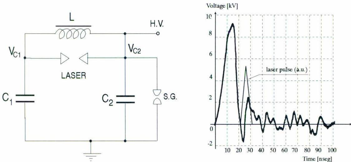
FIGURE 1. (a) Schematic diagram of the Blumlein circuit. (b) Experimentally obtained laser voltage  $V(t)$  and radiation emission at 60 hPa  $N_2$  and H.V. = 8 kV.
