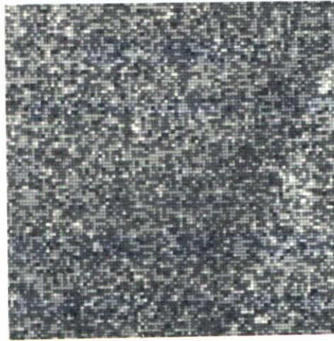
FIGURE 6. Photograph of a 100 \times 100 matrix of random integer values of density written with a microdensitometer. The separation between pixels is 100 \mu\text{m} .
