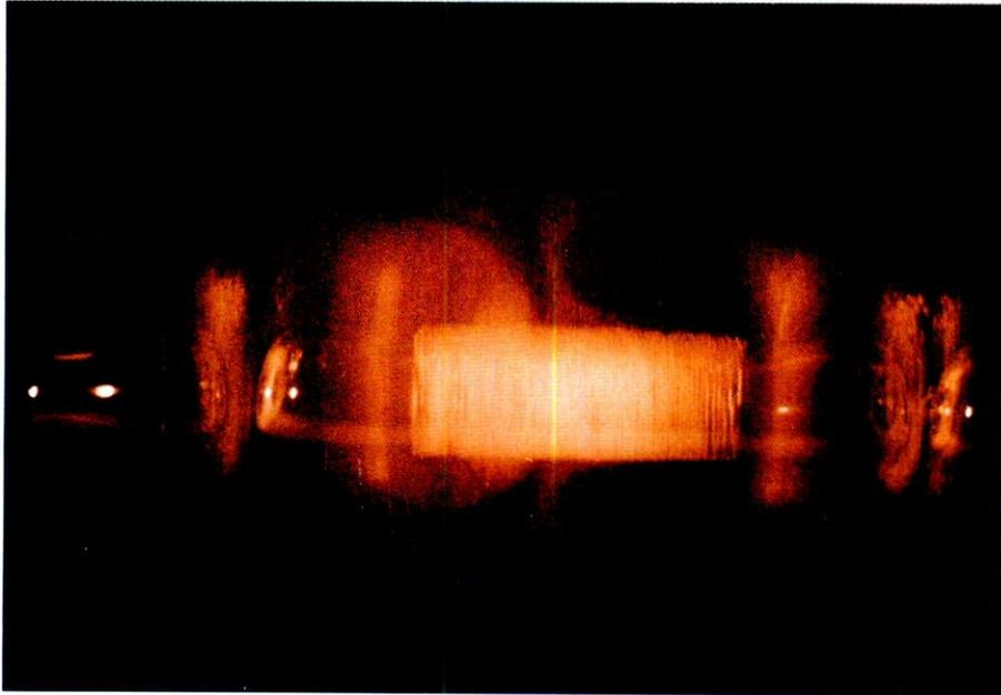
FIGURE 7. Lowering the rotation rate after annular flow has stabilized, leads to pinching of the inner air tube. The small bubbles are trapped in areas with local pressure minima.
