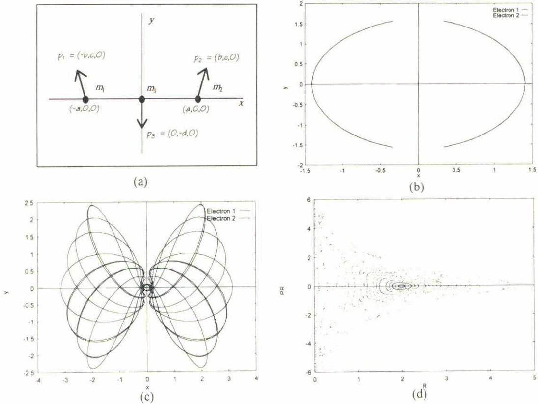
FIGURE 3. Langmuir type orbits in the He atom. (a) Geometry of the initial conditions. (b) Basic orbit (shortest periodic orbit in the He atom). (c) A more complex orbit. (d) Poincaré map of a family of trajectories in hyperspherical coordinates ( $R - P_R$  plot).
