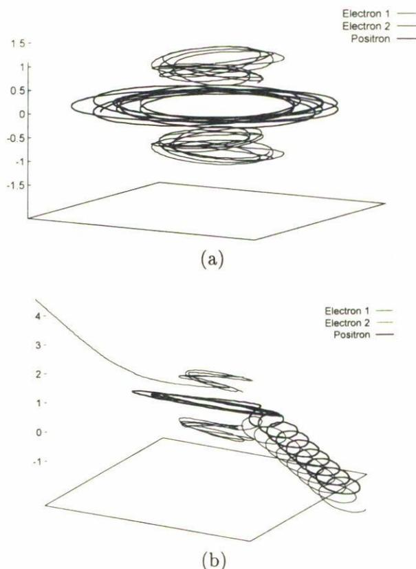
FIGURE 8. Asymmetric top orbits for the  $\text{Ps}^-$  ion. (a) One such orbit. (b) Symmetry-breaking perturbation on the initial conditions, rapidly leading to autoionization.
