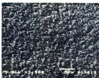
FIGURE 6. Scanning electron microscope picture of the GaAs layer grown with the experimental setup d .
