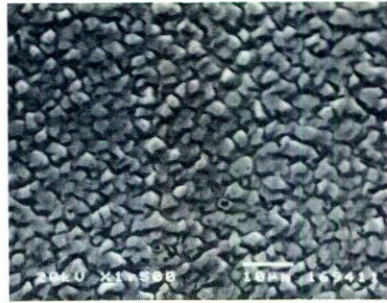
FIGURE 3. A SEM planar view of the homoepitaxial GaAs layer grown with the experimental setup a .
