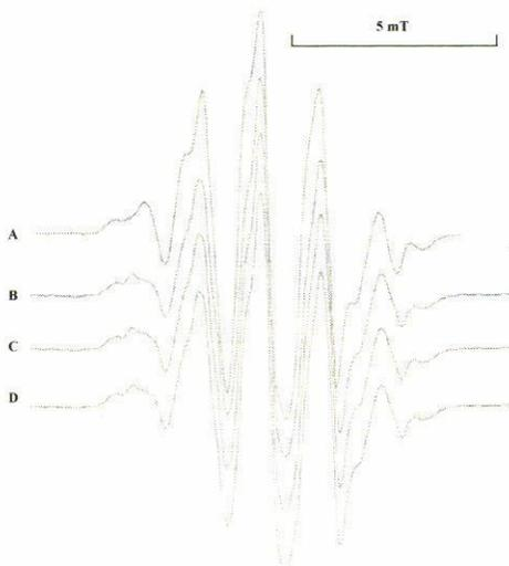
FIGURE 1. First derivative of the ESR spectra of gamma-ray irradiated samples (1 kGy) of (A) AMINOGRAY™, (B) silicone-bound alanine, (C) silicone-bound alanine-boric acid, and (D) silicone-bound alanine-borax. Microwave power 4 mW; modulation amplitude 0.4 mT (100 kHz); time constant 0.3 s.
