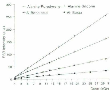
FIGURE 2. Dose response curves for alanine dosimeters gamma-ray irradiated in the 1 to 30 kGy range.
