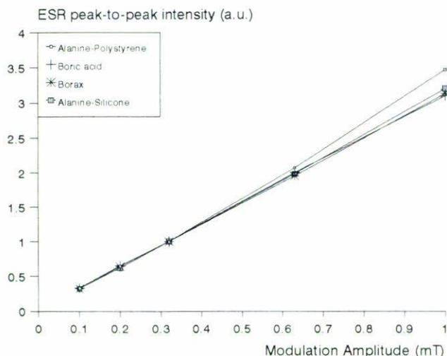
FIGURE 4. Plot of the ESR peak-to-peak intensity as a function of the modulation amplitude for the four types of irradiated dosimeters (1 kGy).
