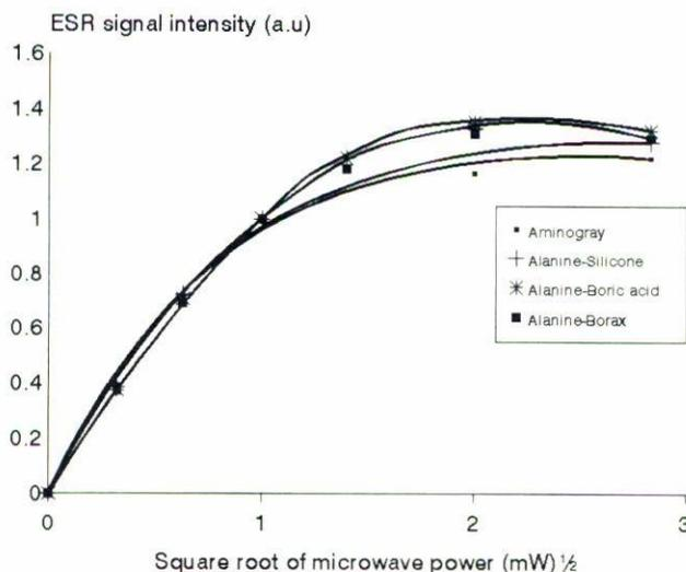
FIGURE 3. Signal amplitude response as a function of the square root of the powder for the four types of irradiated dosimeters (1 kGy).
