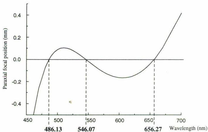
FIGURE 5. Paraxial focal positions plotted against wavelength for the optical system with the parameters of Table III. This configuration is corrected of secondary spectrum by using normal glasses only.
