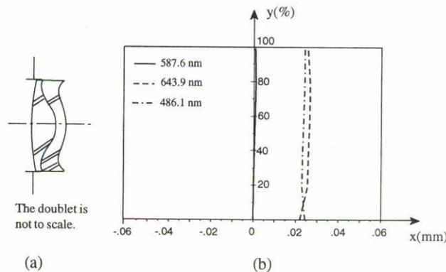
FIGURE 2. (a) Aspheric achromatic doublet, with the parameters of Table I. (b) Longitudinal ray aberrations: 587.6 nm solid line, 643.9 nm dashed line and 486.1 nm dashed line with dots.
