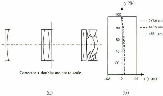
FIGURE 3. (a) Optical system consisting of corrector + aspheric achromatic doublet, with the parameters of Table II. (b) Longitudinal ray aberrations: 587.6 nm solid line, 643.9 nm dashed line and 486.1 nm dashed line with dots.
