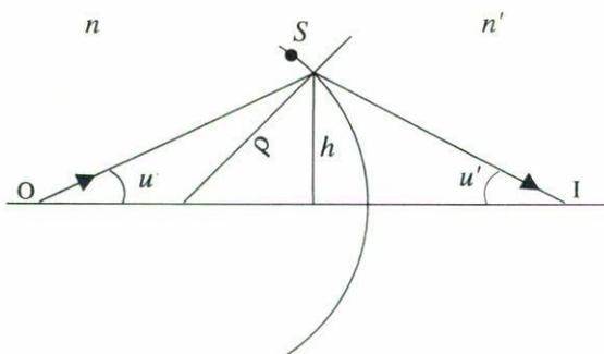
FIGURE 1. Parameters for the evaluation of the Wynne coefficients.
