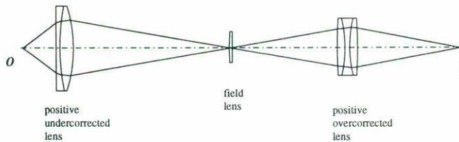
FIGURE 4. Optical system working with an object point at a finite distance. Its parameters are given in Table III. Note that the drawing is not to scale.
