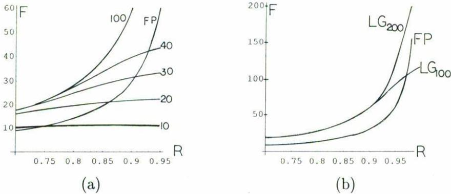
FIGURE 6. (a) Finesse of LG ( $N = 10, 20, 30, 40, 100$ ) and FP interferometers (LGI or side illuminated FPI) compared to the conventional FPI. (b) Finesse of LG ( $N = 100, 200$ ) and FP interferometers.
