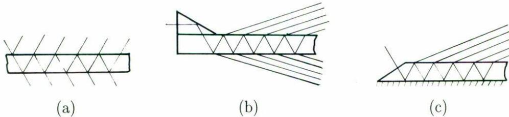
FIGURE 1. Schematic diagram of multiple beam interference in FP (a), and LG (b) and (c) interferometers.
