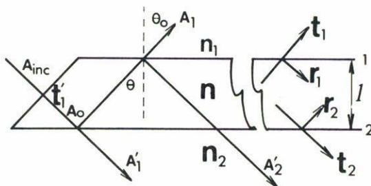
FIGURE 2. Defining the plate parameters.
