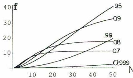
FIGURE 4. The function  $f(N, R)$ , Eq. (13), of LGI vs. the number reflections  $N < 50$  at different values of the reflection coefficient  $R = 0.7, 0.8, 0.9, 0.95, 0.99, 0.999$ .
