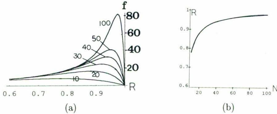
FIGURE 5. (a) The function  $f(N, R)$  of LGI vs. the reflection coefficient  $R$  at a given number of reflections  $N(= 10, 20, 30, 40, 50, 100)$ . (b) The optimal value of the reflection coefficient  $R$  for different numbers of reflection  $N$  inside LGI.
