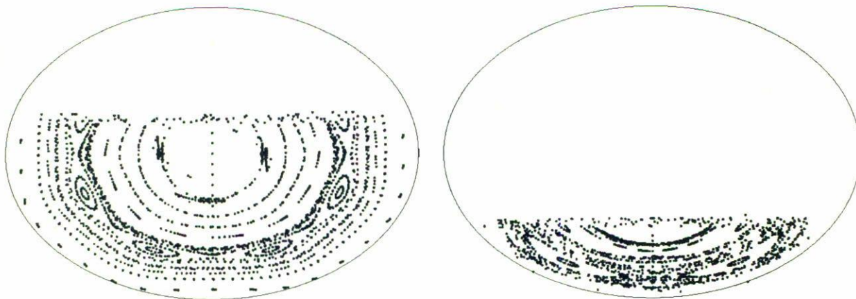
FIGURE 8. Chaotic advection in ellipses of aspect ratio 0.7 in the continuous flow regime. Different fill levels are shown. The right figure displays an unmixed central core (J. Gilchrist, in progress)
