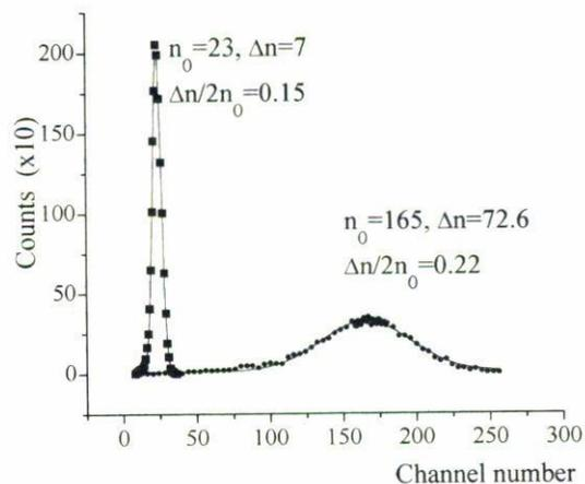
FIGURE 3. Example of two different experimental distributions of laser pulse energy with the parameters of the fitted Gaussian.
