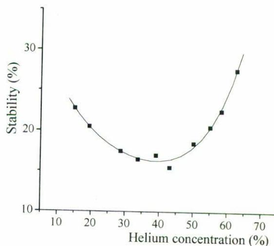
FIGURE 7. Laser output stability ( $\Delta n/2n_0$ ) vs. percentage of He in the gas mixture.
