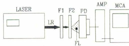
FIGURE 2. Experimental set-up schematic diagram. LR is the laser radiation, F1 and F2 are the ultraviolet and fluorescing filters, FL is the fluorescence, PD is the photodiode, AMP is the amplifier and MCA is the multichannel analyzer.
