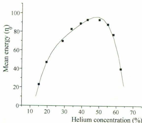
FIGURE 6. Central channel position ( $n_0$ ) vs. percentage of He in the gas mixture.
