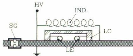
FIGURE 1. Experimental arrangement of the  $N_2$  laser. SG is the spark gap, IND is the uncoupling inductance, LC is the laser camera, LE are the laser electrodes and HV is the high voltage.
