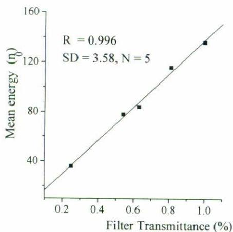
FIGURE 4. Central channel position ( $n_0$ ) vs. attenuation of the laser radiation.
