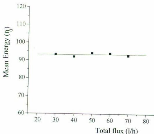
FIGURE 5. Central channel position ( $n_0$ ) vs. 1:1 gas mixture flux.
