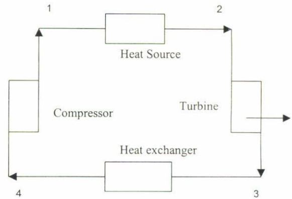
FIGURE 3. Basic components of the closed gas-turbine.
