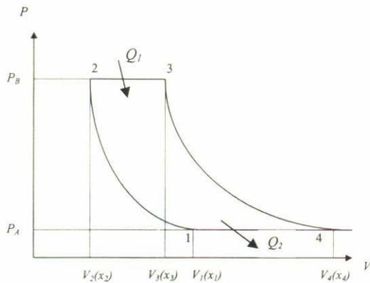
FIGURE 2. Pressure-volume diagram of the Joule-Brayton cycle.  $V_i$  ( $i = 1, 2, 3, 4$ ) correspond to displacements  $x_i$  ( $i = 1, 2, 3, 4$ ). The relation between  $V_i$  and  $x_i$  is  $V_i = Ax_i$  where  $A$  is the cross section.
