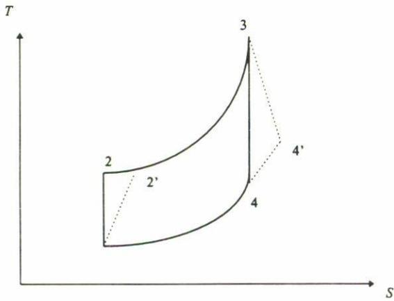
FIGURE 1. Temperature-entropy diagram of the cycle.
