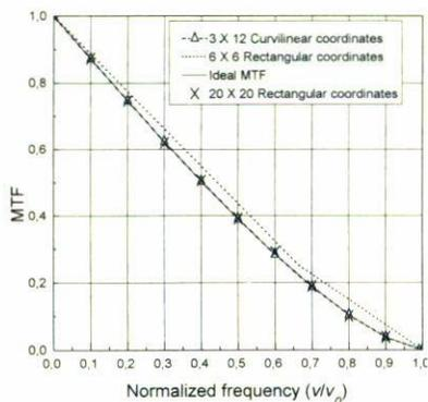
FIGURE 8. Modulation transfer function versus normalized frequency,  $v/v_0$ , for an aberration-free system in focus.
