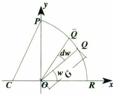
FIGURE 6. Geometry for the derivation of  $dw/dv$ .
