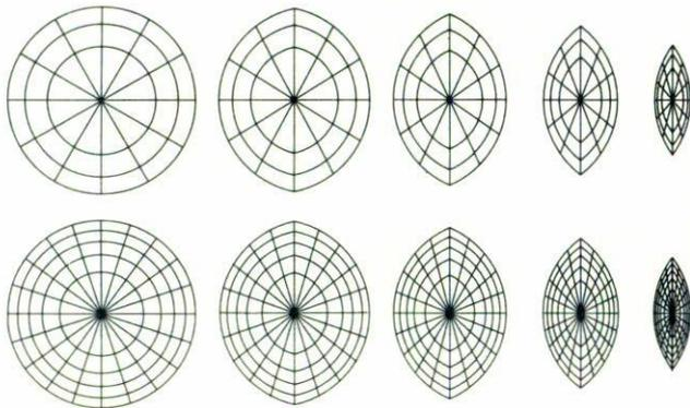
FIGURE 7. Domain of integration divided into 3 rings and 12 sectors (upper row) and 5 rings and 20 sectors (lower row) for normalized frequencies of 0%, 20%, 40%, 60% and 80% from left to right.
