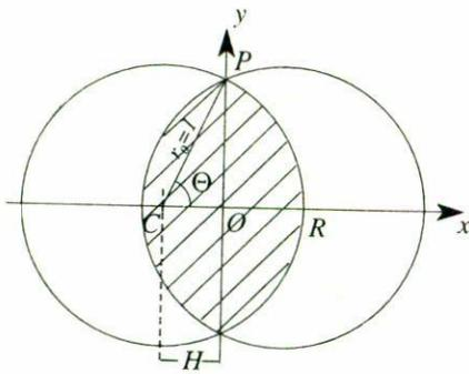
FIGURE 1. The domain of integration,  $S$ , which is denoted by the dash area, is defined by shearing the pupil an amount proportional to the spatial frequency
