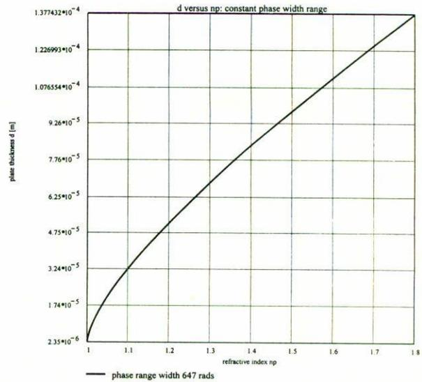
FIGURE 4. Thickness  $d$  as a function of the refractive index  $n_p$  for the case of a phase width range  $\Phi_w$  value of 647 rads (solid line). The plot really begins at  $n_p = 1.01$ .
