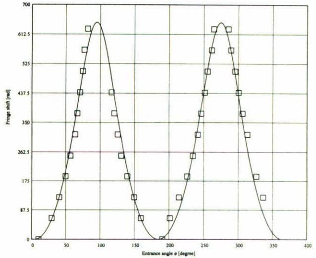
FIGURE 3. Experimental data (squares) obtained with the interferometer of Fig. 2. Preliminary data fitting of  $\Delta\Phi(\phi)$  for the data set [Eq. (5)]: assuming  $d = 6 \times 10^{-5}$  m, the fitting gives  $n_p = 1.248$ ,  $\Phi_w = 647.62$  rads, and  $\Delta\phi = -4.223^\circ$ .
