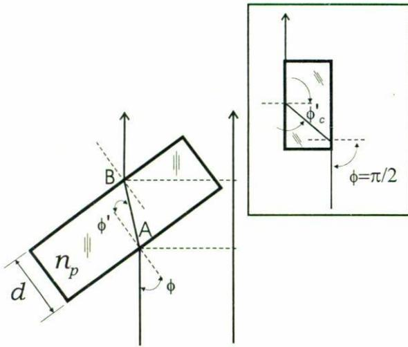
FIGURE 1. Determination of the OPD as a function of the entrance angle  $\phi$ .  $\phi'$  is the refracting angle,  $n_p$  the plate's refractive index, and  $d$  its thickness. Inserted figure: grazing incidence case.  $\phi'_c$  is the critical angle.
