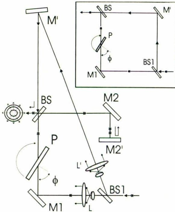
FIGURE 2. Experimental arrangements used for fringe counting. P: transparent parallel plate, M1, M2, M', M2': mirrors, L, L': beam expander/collimating systems, BS1: entrance beam splitter, BS: output beam splitter. Similar notation is employed in the insert.
