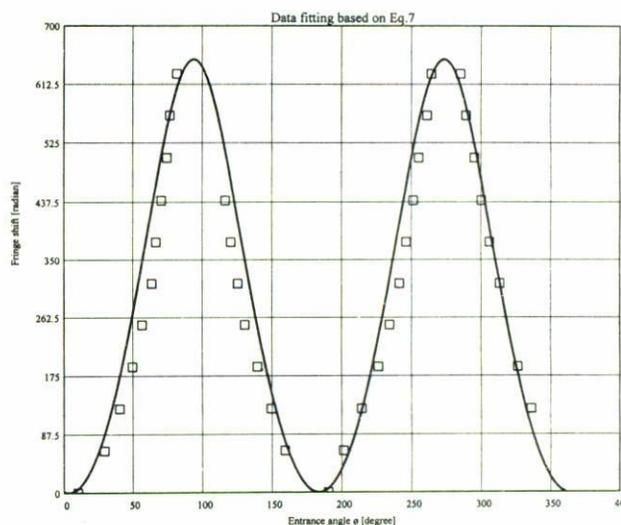
FIGURE 6. Fitting using Eq. 7 and first assuming  $\Phi_w = 650$  rads. This gives  $\Phi_w = 649.844$  rads,  $n_p = 1.529$  and  $\Delta\phi = -3.299^\circ$ . The calculation of the thickness gives  $d = 1.025 \times 10^{-4}$  m, while  $\Phi_{max} = 2.667 \times 10^3$  rads and  $\Phi_{min} = 2.017 \times 10^3$  rads.
