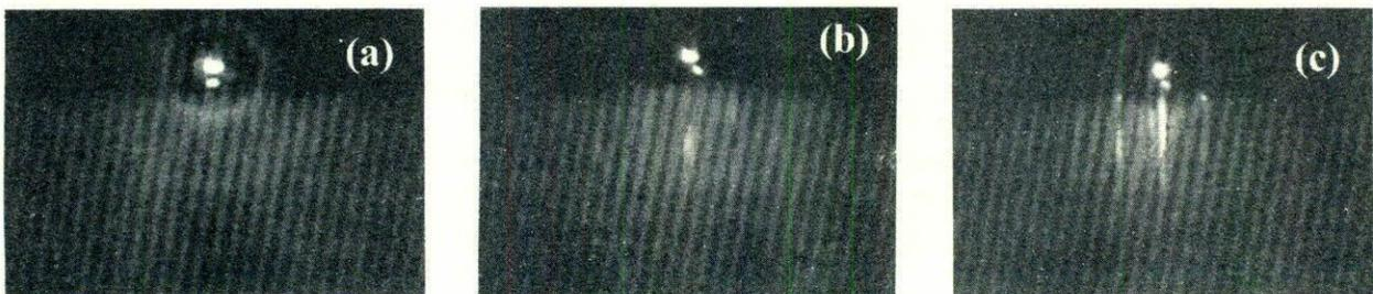
FIGURE 6. RHEED patterns of: (a) the initial as-loaded GaAs(100) surface, (b) the GaAs surface after the outgassing process at 350°C, (c) the GaAs surface after the removal of the oxides at a temperature of 530°C.
