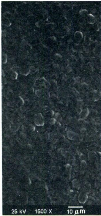
FIGURE 4. SEM microstructure of the CdTe film (9,8 μm) deposited by DCSVT on the ITO substrate (CdTe/ITO/glass) under the following conditions: T(\text{source}) = 660^\circ\text{C} , T(\text{substrate}) = 585^\circ\text{C} , P(\text{O}_2) = 2 \text{ mbar} , P(\text{He}) = 14 \text{ mbar} , time = 4 min.
