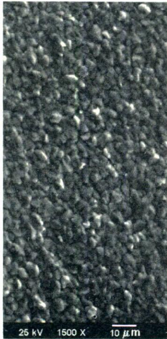
FIGURE 5. SEM microstructure of the CdTe film (16 μm) deposited by DCSVT on the CdS substrate (CdTe/CdS/ITO/glass) under the following conditions: T(\text{source}) = 650^\circ\text{C} , T(\text{substrate}) = 590^\circ\text{C} , P(\text{O}_2) = 2 \text{ mbar} , P(\text{He}) = 14 \text{ mbar} , time = 4 min.
