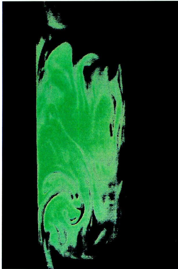
FIGURE 3. Volutes inherent to a turbulent natural convection mixing process of two fluids of different density inside a cylindrical cavity.
