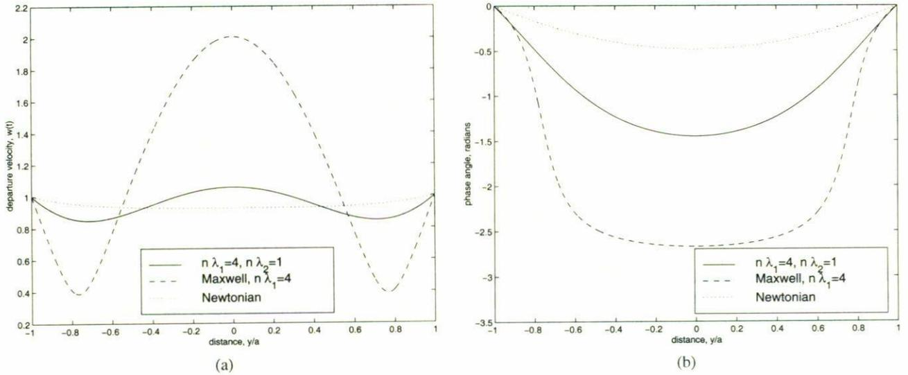
FIGURE 1. Parallel planes: (a) velocity departure from the steady state value vs. distance and (b) phase angle of velocity departure vs. distance between the planes for an Oldroyd fluid with  $n\lambda_1 = 4, n\lambda_2 = 1$ . The Maxwell model with  $n\lambda_2 = 0$  and the Newtonian fluid are shown for comparison.
