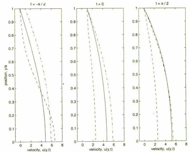
FIGURE 6. Parallel planes: velocity profiles at various times. The  $z$  axis is located midway between the planes. Oldroyd fluid with  $n\lambda_1 = 20, n\lambda_2 = 2$  - - - -; Maxwell model .....; Newtonian - . - . - .
