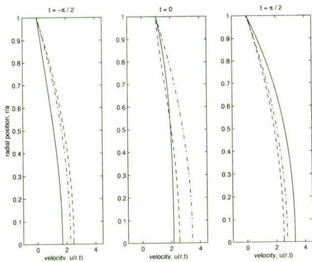
FIGURE 5. Pipe flow: velocity profiles at various times. The  $z$  axis is located at the center of the pipe. Oldroyd fluid with  $n\lambda_1 = 20, n\lambda_2 = 2$  - - - -; Maxwell model .....; Newtonian - . - . - .
