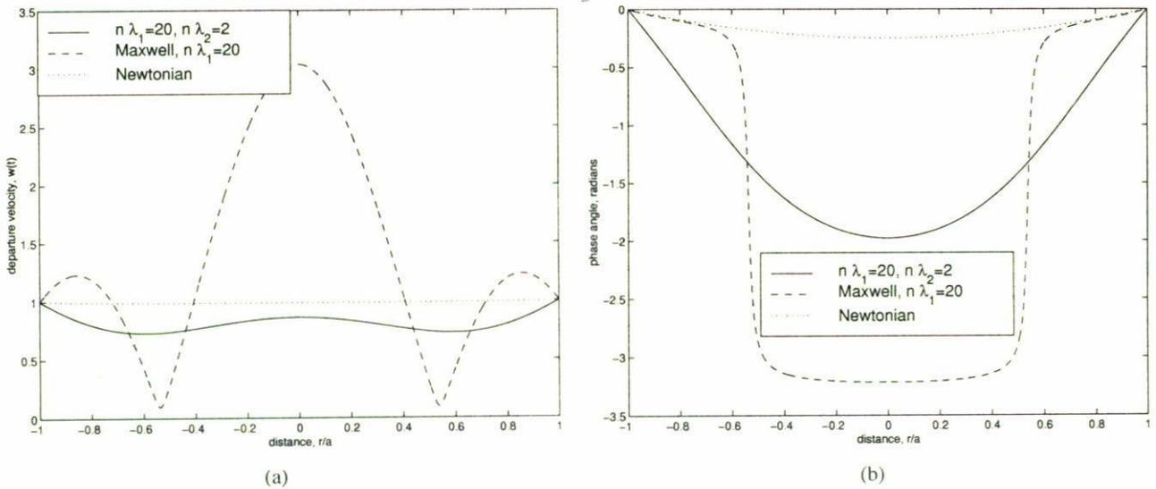
FIGURE 4. Pipe flow: velocity departure from the steady state value vs. radial distance and (b) phase angle of velocity departure vs. radial distance for an Oldroyd fluid with  $n\lambda_1 = 20, n\lambda_2 = 2$ . The Maxwell model with  $n\lambda_2 = 0$  and the Newtonian fluid are shown for comparison.
