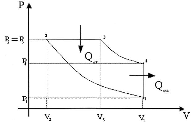
FIGURE 2 Pressure-volume diagram of an ideal Diesel cycle.
