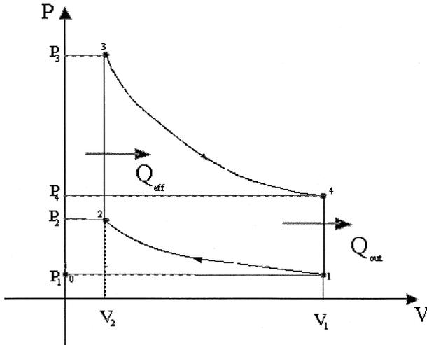
FIGURE 1 Pressure-volume diagram of an ideal Otto cycle.
