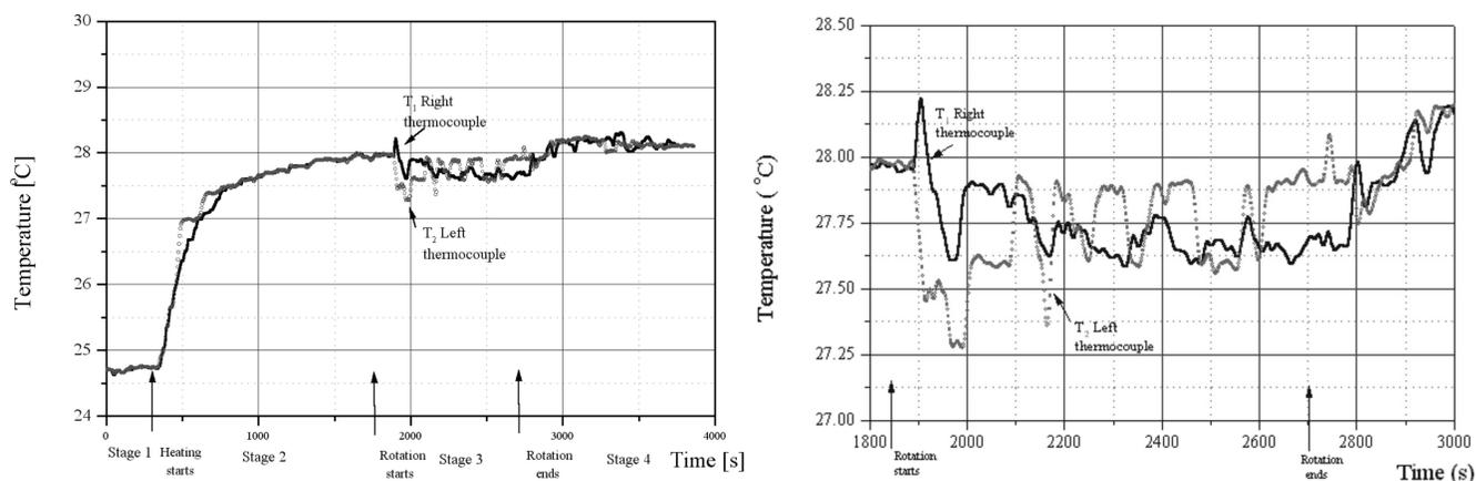
FIGURE 11. Temperature as a function of time a) during a sample experiment with four different stages. and b) amplification of the stage 3,  $Ra_r = 3.25 \times 10^6$ ,  $Pr = 6$ , and  $Ta = 1.71 \times 10^7$ .
