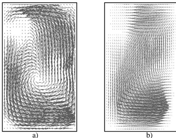
FIGURE 12. Convective flows a) in the nonrotating cavity,  $Ra = 2.25 \times 10^6$ ,  $Pr = 6$ ,  $Ta = 0$  and  $t = 1380$  s. and b) in rotating cavity,  $Ra_r = 3.25 \times 10^6$ ,  $Pr = 6$ ,  $Ta = 1.71 \times 10^7$  and  $t = 1920$  s.
