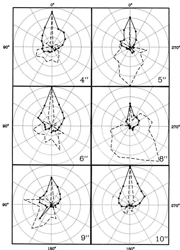
FIGURE 5. Polar coordinate graph of the differential count rate  $[(N_B - N_{BG}) / N_{LC}]$  for 4,5,6,8,9 and 10 inch spheres in the central position for the moderated neutron source. Filled lines were taken without the Cd shell, whereas, dashed lines represent the data from the spheres with the Cd inserted in the radial holes. Not in scale.
