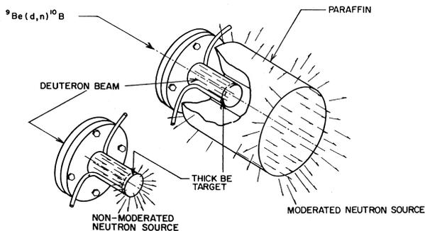
FIGURE 2. Schematic view of the target assembly used.
