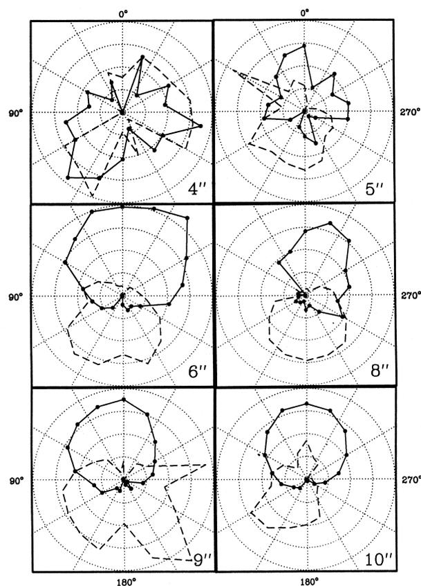
FIGURE 6. Polar coordinate graph of the differential count rate  $[(N_B - N_{BG}) / N_{LC}]$  for 4,5,6,8,9 and 10 inch spheres in the central position for the non-moderated neutron source. Filled lines were taken without the Cd shell, whereas, dashed lines represent the data from the spheres with the Cd inserted in the radial holes. Not in scale.
