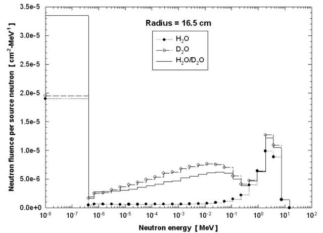
FIGURE 7. Neutron spectra, at 27 cm, produced by a <sup>239</sup>PuBe neutron source inserted at the center of 16.5-cm-radius moderator media (H<sub>2</sub>O, D<sub>2</sub>O and H<sub>2</sub>O/D<sub>2</sub>O).
