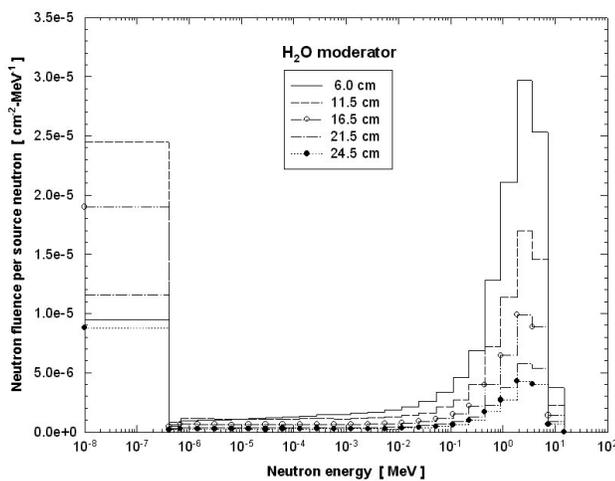
FIGURE 3. Neutron spectra, at 27 cm, produced by a  $^{239}\text{PuBe}$  neutron source inserted at the center of a set of 6.0, 11.5, 16.5, 21.5 and 24.5-cm-radii  $\text{H}_2\text{O}$  moderator media.
