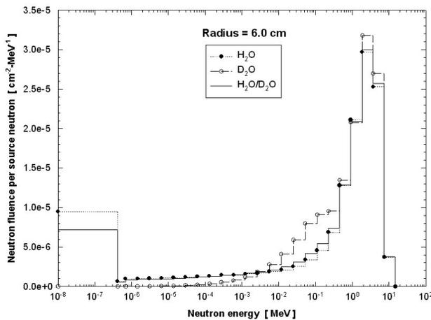
FIGURE 6. Neutron spectra, at 27 cm, produced by a <sup>239</sup>PuBe neutron source inserted at the center of 6.0-cm-radius moderator media (H<sub>2</sub>O, D<sub>2</sub>O and H<sub>2</sub>O/D<sub>2</sub>O).
