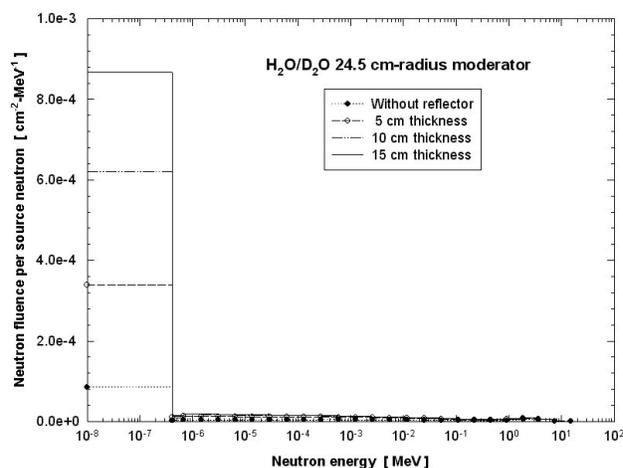
FIGURE 9. Neutron spectra, at 27 cm, produced by a  $^{239}\text{PuBe}$  neutron source inserted at the center of  $\text{H}_2\text{O}/\text{D}_2\text{O}$  24.5-cm-radius moderator, without and with graphite reflector (5, 10, and 15-cm-thickness).
