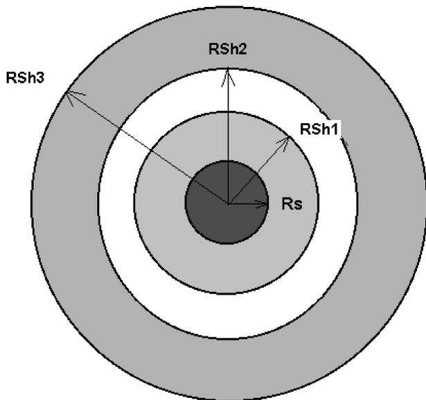
FIGURE 1. Moderator model.  $R_s$  is the source radius (1.0 cm),  $R_{Sh1}$  is the first shell radius (1.5 cm) filled with air,  $R_{Sh2}$  is the second shell radius (5.0 cm) filled with moderator and  $R_{Sh3}$  radius (6.0, 7.0, 11.5, 16.5, 21.5 and 24.5 cm) filled with moderator.
