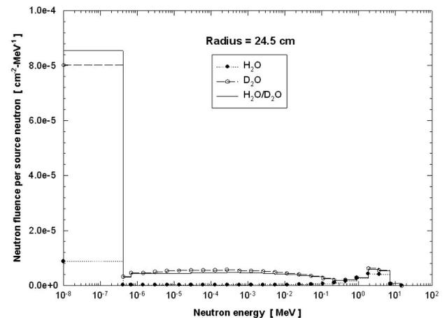
FIGURE 8. Neutron spectra, at 27 cm, produced by a <sup>239</sup>PuBe neutron source inserted at the center of 24.5-cm-radius moderator media (H<sub>2</sub>O, D<sub>2</sub>O and H<sub>2</sub>O/D<sub>2</sub>O).
