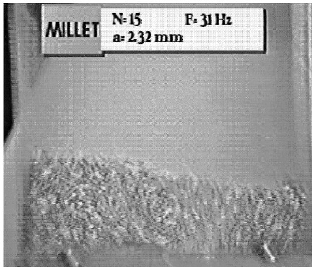
FIGURE 4. On the left side, a heap develops even for \Gamma < 1 . Significant lateral waves and arching exist under 30^\circ combined vibration. A single convection cell is observed for values greater than \Gamma=8.97 .
