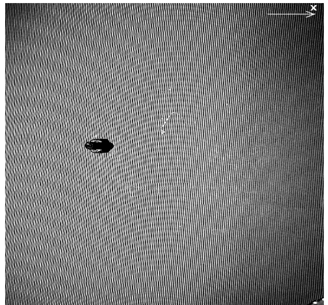
FIGURE 4. A typical image used in the calculation of the optical phase.
