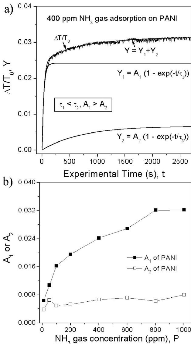
FIGURE 2. a) Fitting of the kinetic adsorption curve of PANI film exposed to 400 ppm NH<sub>3</sub> gas in Fig. 1c. b) Fitting parameters A<sub>1</sub> and A<sub>2</sub> of the PANI single film based optochemical gas sensor as a function of NH<sub>3</sub> gas concentration.
