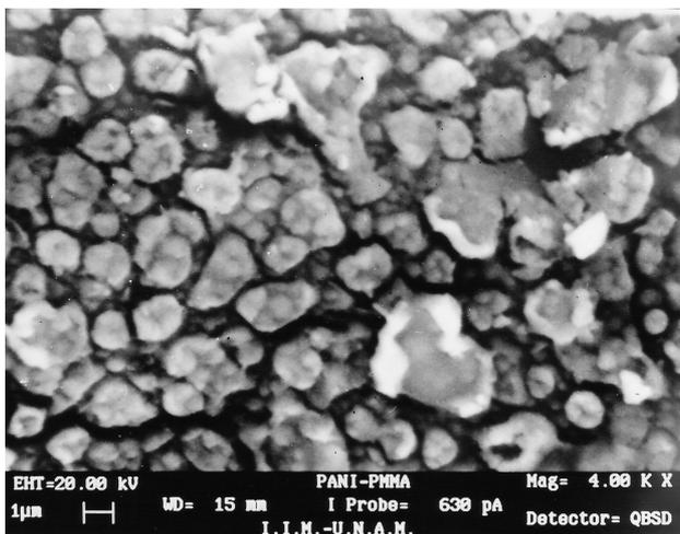
FIGURE 6. SEM micrograph of a PANI-PMMA sample, with 5 wt% aniline in the composite film.
