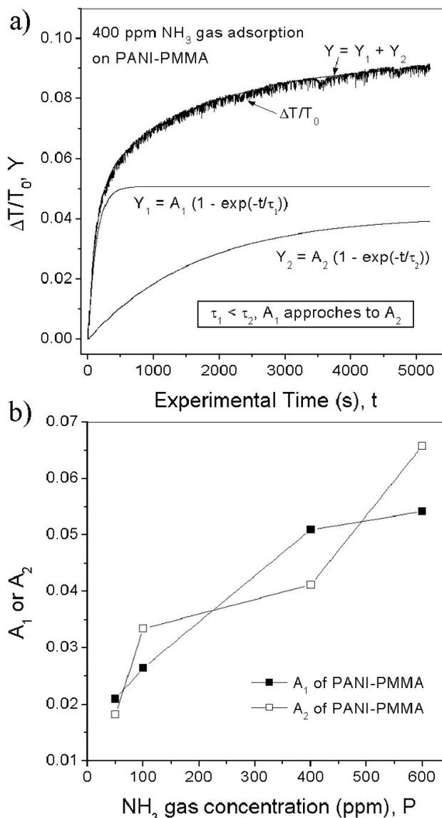
FIGURE 3. a) Fitting of the kinetic adsorption curve of PANI-PMMA film exposed to 400 ppm NH<sub>3</sub> gas in Fig. 1c. b) Fitting parameters A<sub>1</sub> and A<sub>2</sub> of the PANI-PMMA composite film based optochemical gas sensor as a function of NH<sub>3</sub> gas concentration.
