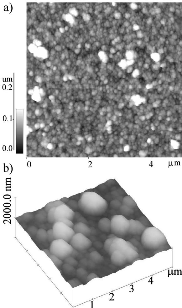
FIGURE 5. AFM micrograph of: a) a polyaniline thin film sample, deposited at 5°C, showing a porous and granular surface morphology. b) a P3MT thin film sample, prepared by the electrochemical method.
