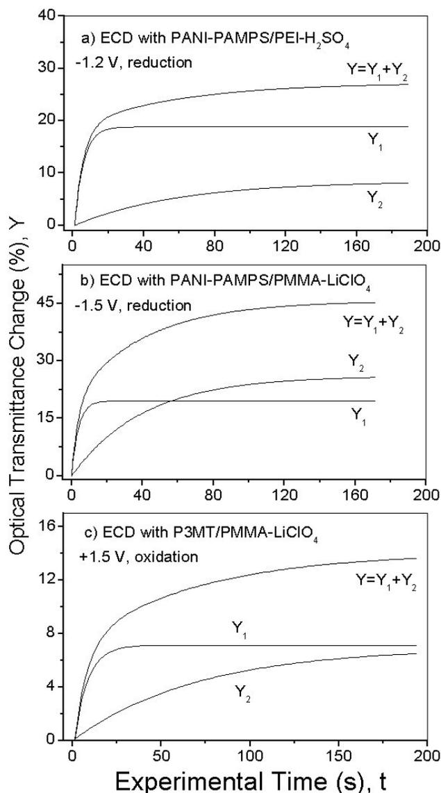
FIGURE 4. Fitting of the optical transmittance changes of ECDs as a function of experimental time: a) at 632 nm of PANI-PAMPS based device with PEI- $\text{H}_2\text{SO}_4$  as solid electrolyte; b) 632 nm of PANI-PAMPS based device with PMMA- $\text{LiClO}_4$  as solid electrolyte; c) at 550 nm of P3MT based device with PMMA- $\text{LiClO}_4$  as solid electrolyte.
