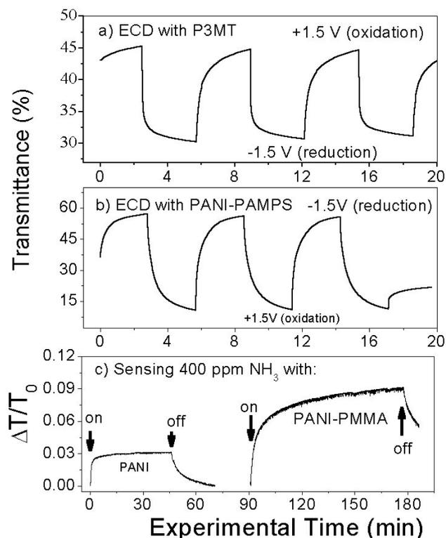
FIGURE 1. Kinetic optical transmittance curves (a) at 550 nm of P3MT based ECD with PMMA-LiClO<sub>4</sub> as solid electrolyte, and (b) at 632 nm of PANI-PAMPS based ECD with PMMA-LiClO<sub>4</sub> as solid electrolyte. (c) Optical transmittance change ( $\Delta T/T_0$ ) at 632 nm of PANI and PANI-PMMA films as they are exposed to 400 ppm NH<sub>3</sub> gas.
